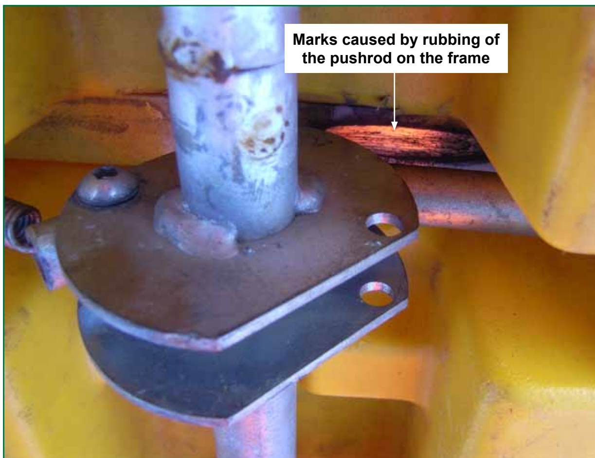
Figure D9: Close-up of the upper brake pushrod, showing evidence of rubbing on the frame
