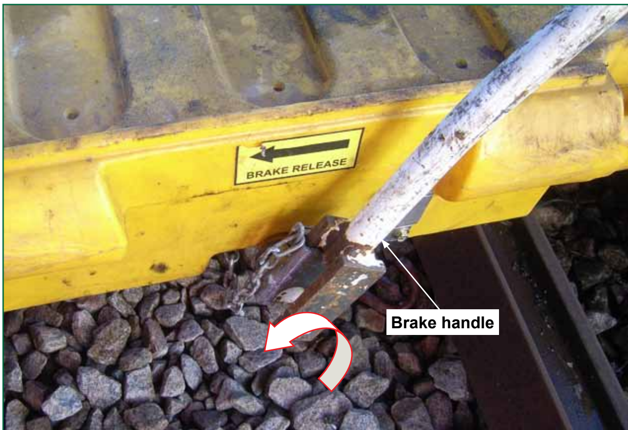
Figure D2: One end of 'trakrat' LT1000P, showing use of brake handle to release brakes
