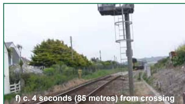
Figures 10a to 10f: Views from the south side of Mexico footpath crossing towards a train approaching from the east taken at 1.45 metres above ground level and at 2 metres from the nearer rail. The images show that although part of the train is always in view, the distinctive marker light at the front of the train is temporarily hidden by the equipment cases at 7 seconds from the crossing and by the signal post at 4 seconds from the crossing.
