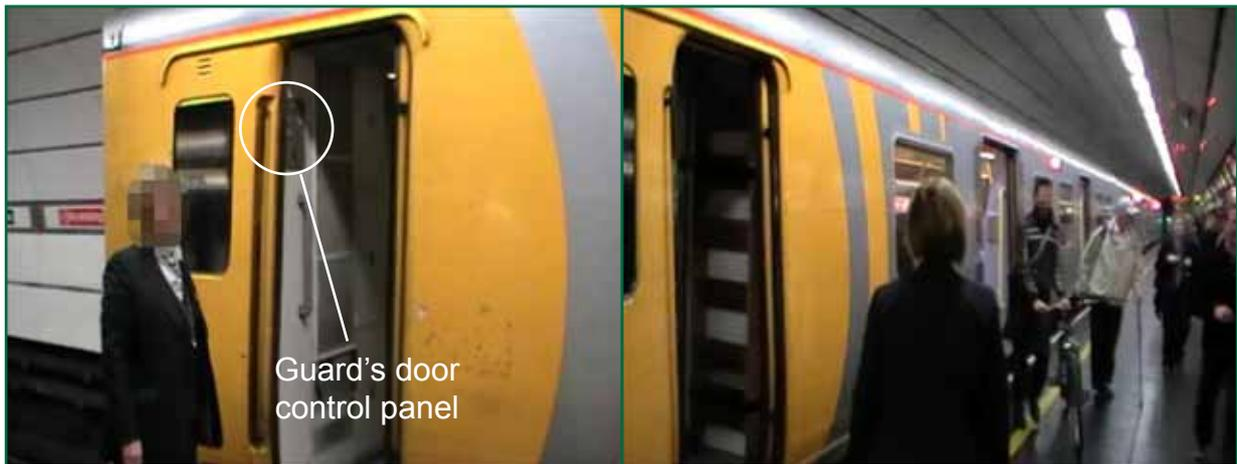
Figure 7: A guard carrying out a safety check
