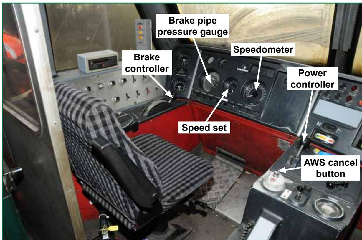
Figure 5: Layout of cab controls, class 90 locomotive
