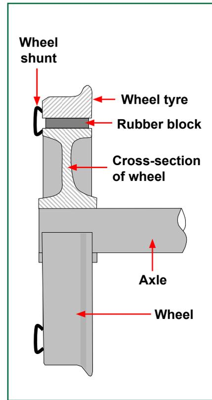
Figure 14: Part-section of wheel
