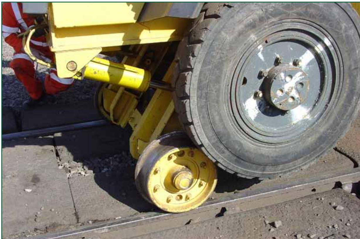
Figure 3: Rear rail axle in fully lowered position
