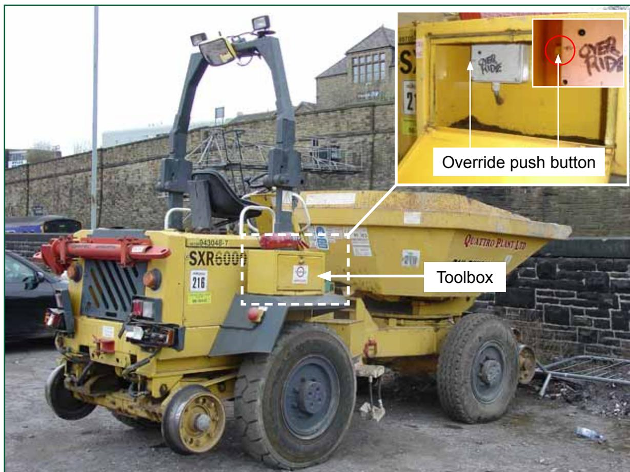
Figure 7: Location of interlock circuit box and override button
