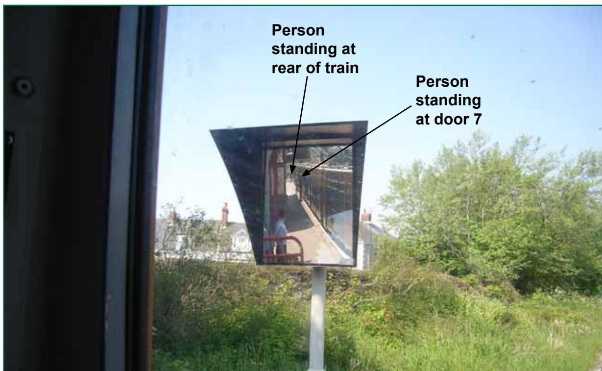
Figure 9: Typical view of the platform/train interface from the driver's cab through the mirror on platform 2 at Jarrow station (Note that the station canopy shadow at the time of the incident would not have been so pronounced)
