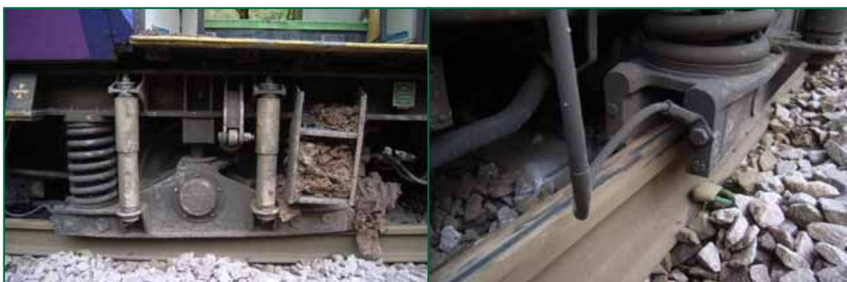
Figure 3: Detail of the axlebox on derailed train 2R15 engaging with the rail
