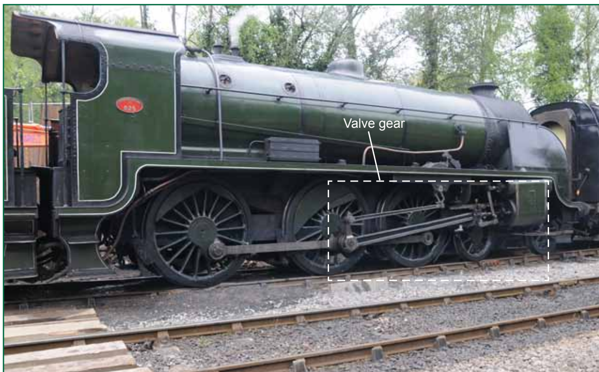
Figure 5: Valve gear fitted to S15 class locomotive no.825 with the locomotive in reverse gear
