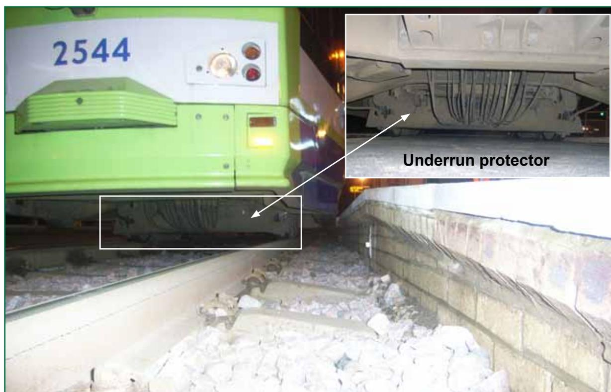
Figure 7: Front of tram showing underrun protector
