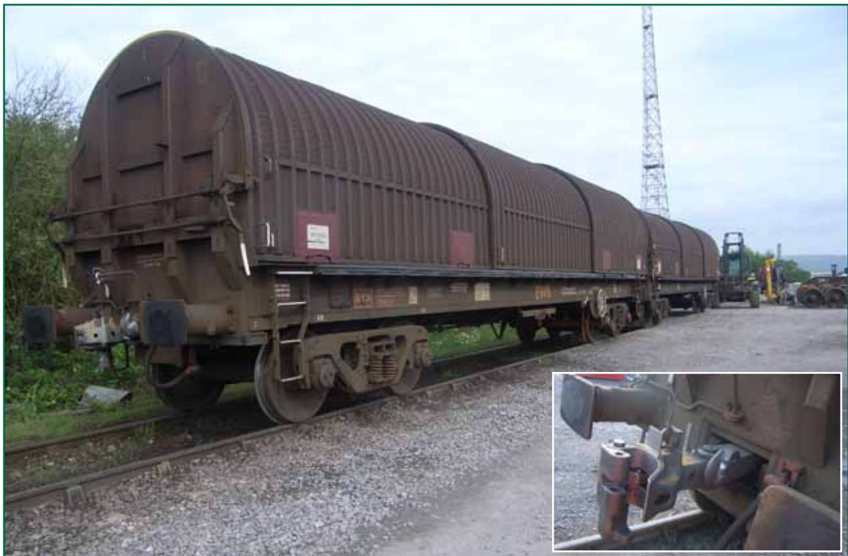
Figure 1: Incident wagons with buckeye coupler
