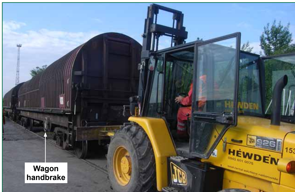
Figure 2: Adapted forklift and wagon handbrake
