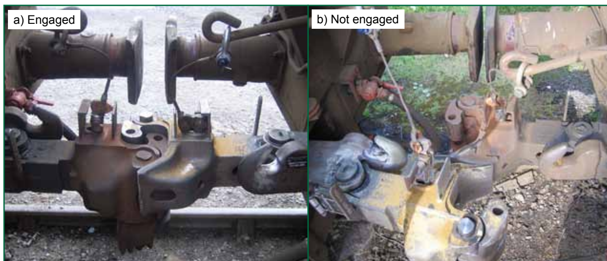
Figure 7: Buckeye coupling engagement
