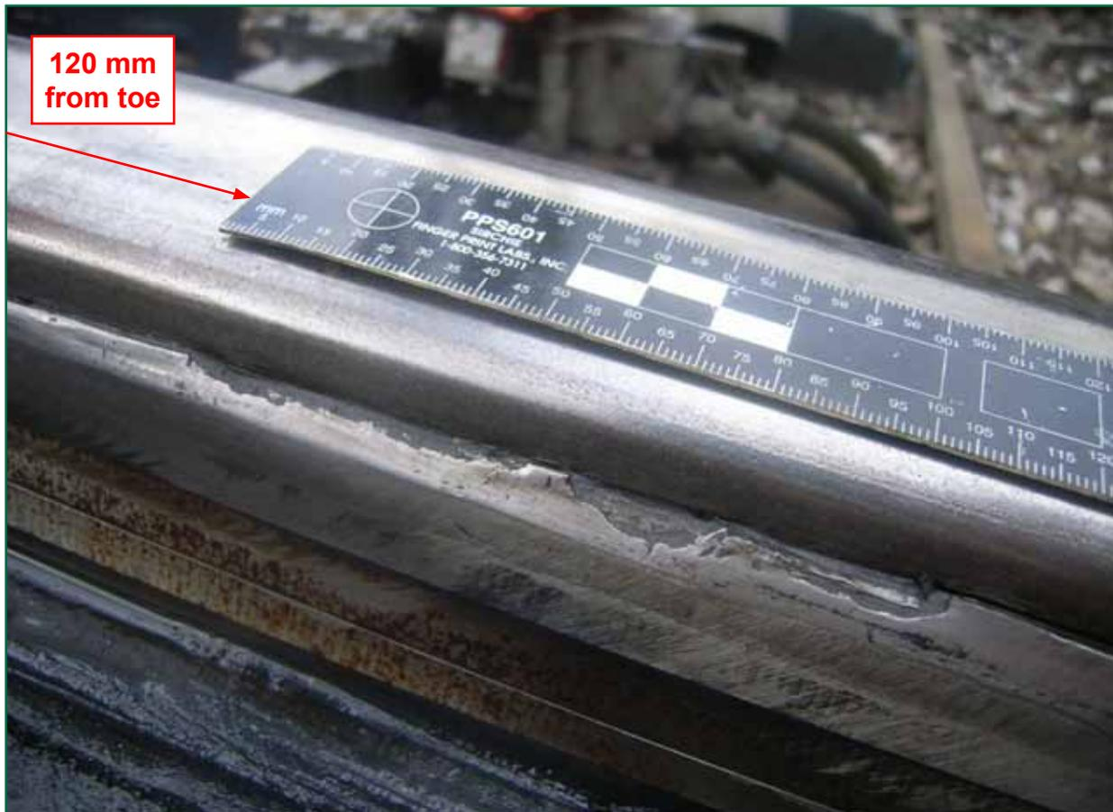
Figure 7: Left-hand switch rail damage
