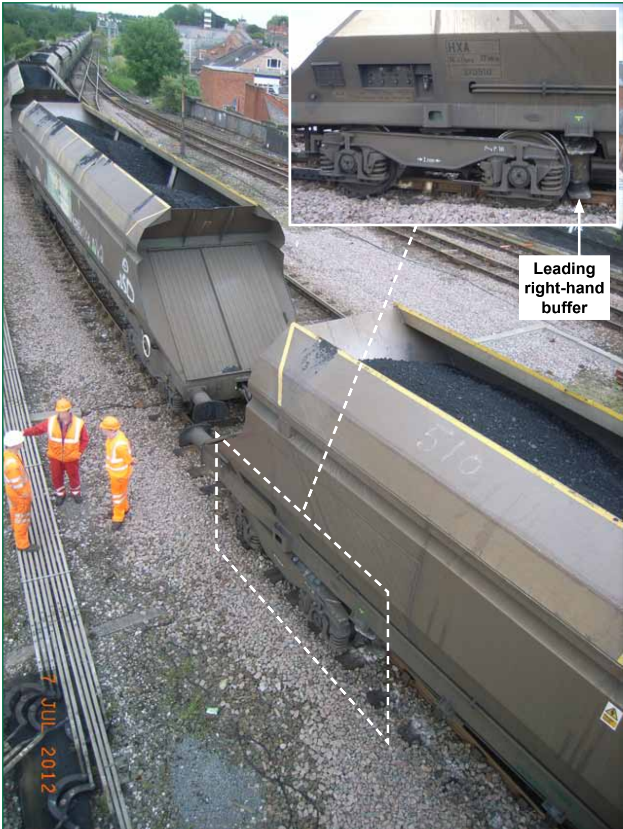
Figure 2: Wagon 370510 after the derailment
