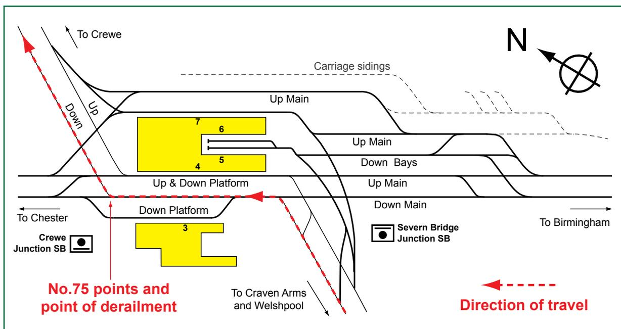
Figure 3: Schematic diagram showing location of accident
