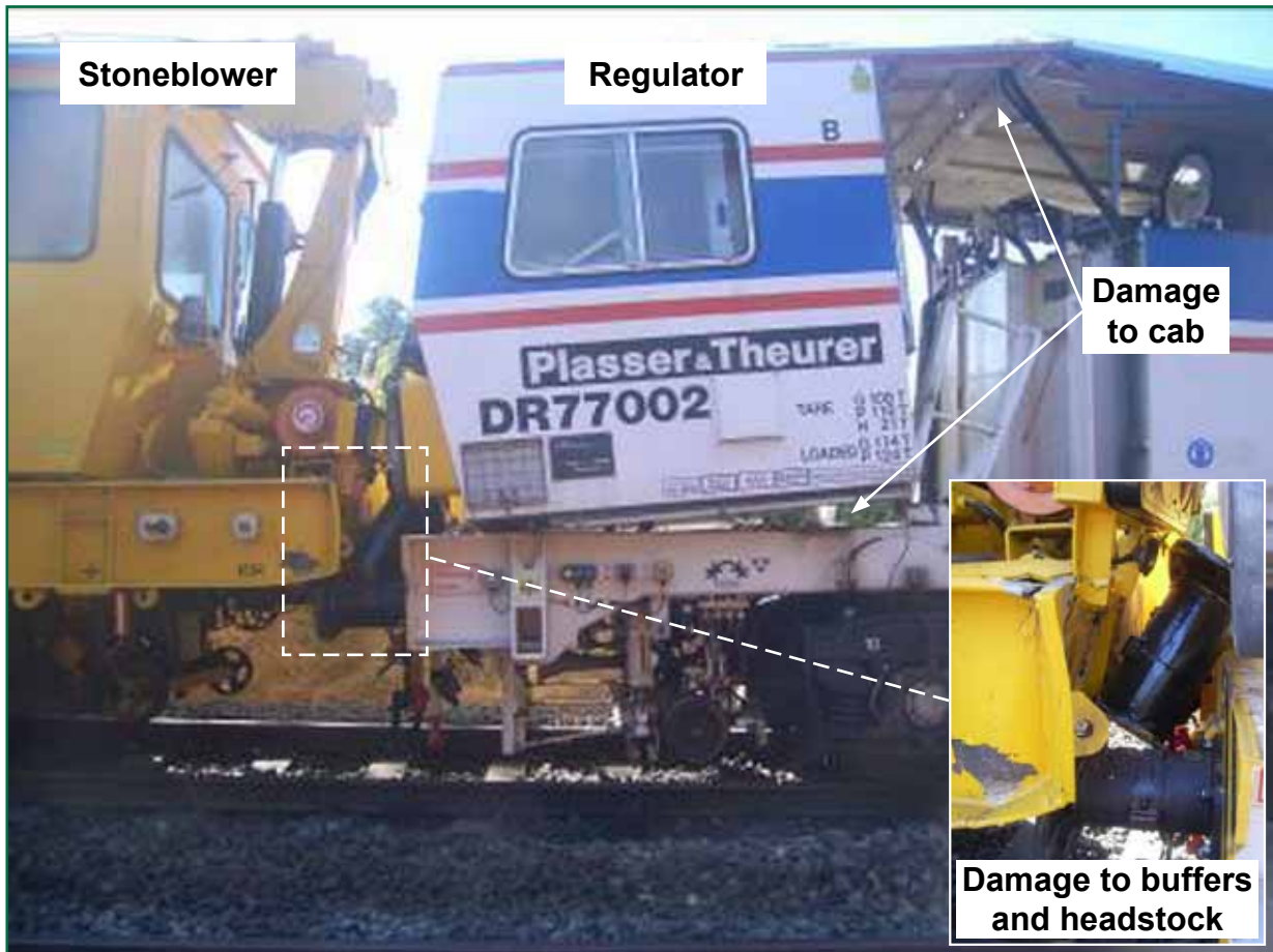
Figure 3: Damage to stoneblower and regulator caused by the collision
