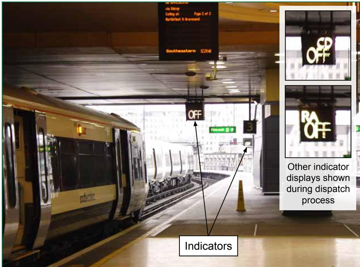
Figure 4: Dispatch indicators on Charing Cross platform 3
