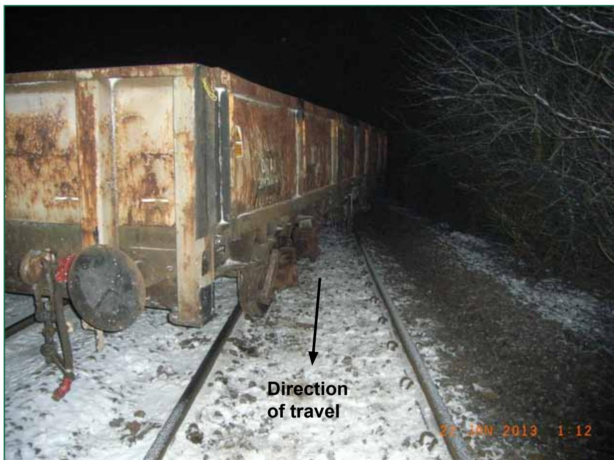
Figure 7: The rearmost derailed wagon (the twentieth wagon) which ended up foul of the down Chellaston line
