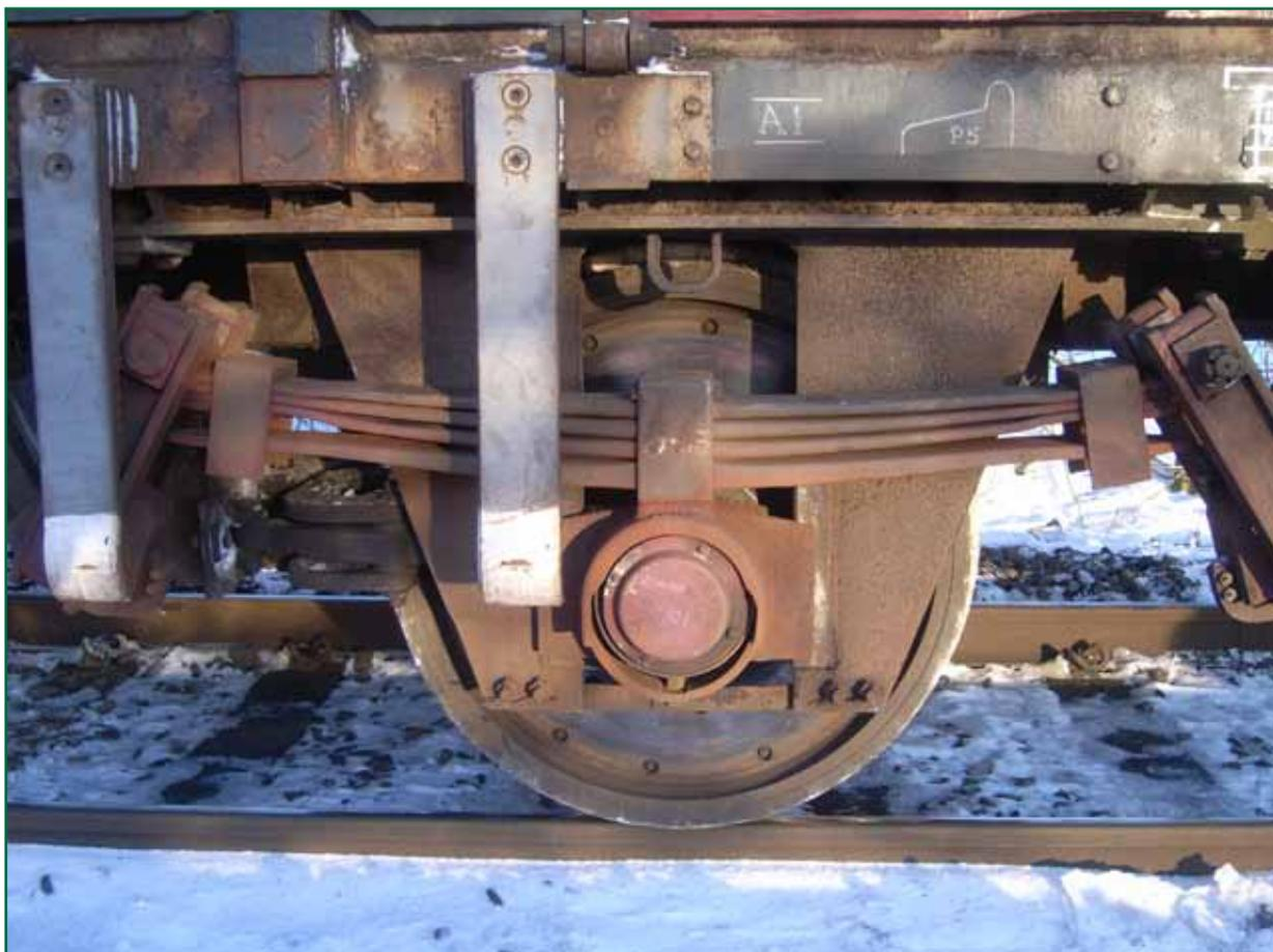
Figure 6: Parabolic leaf spring suspension
