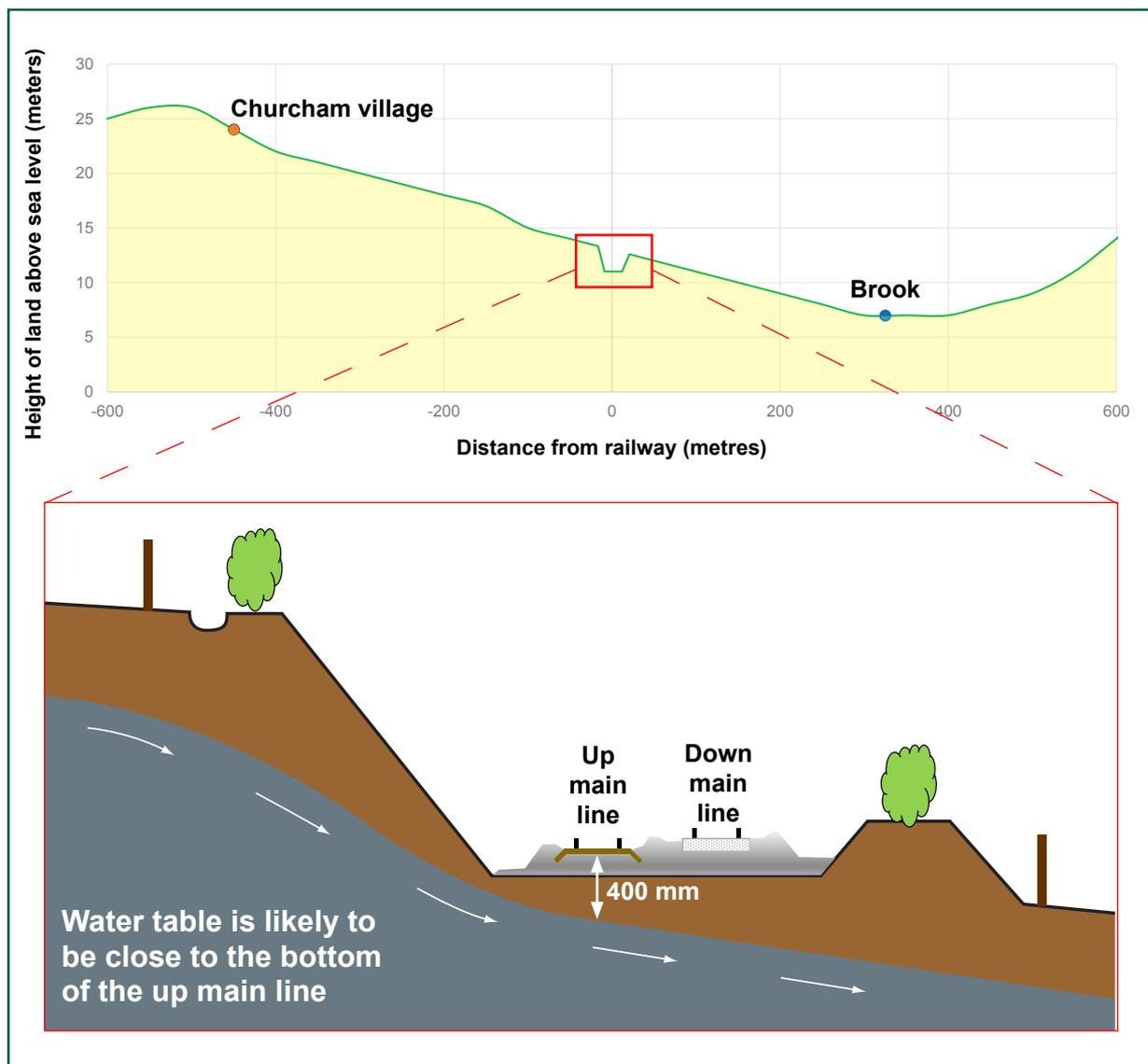
Figure 13: Profile of the land perpendicular to the railway and side view of the cutting
