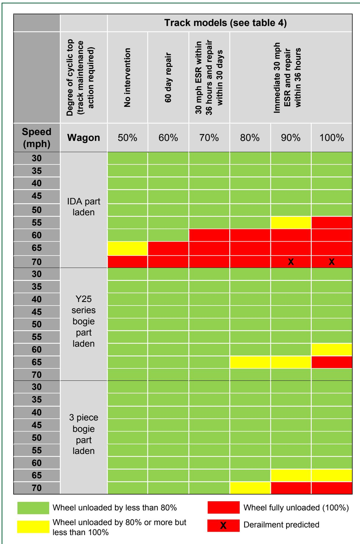
Figure 26: Simulation results for different wagons in their part laden condition
