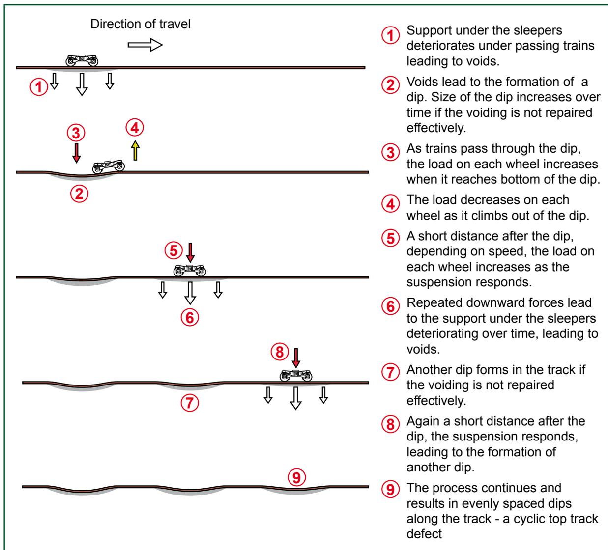
Figure 17: Formation of a cyclic top track defect
