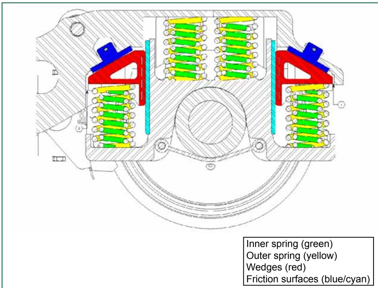
Figure 23: The primary suspension on an IDA wagon
