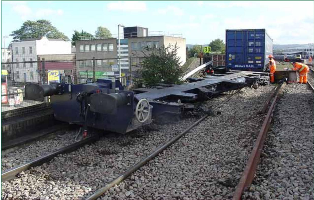
Figure 8: The severely damaged vehicle at the rear of train 4M36
