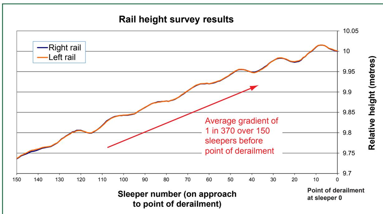
Figure 10: Graph showing the changes in vertical height of the rails
