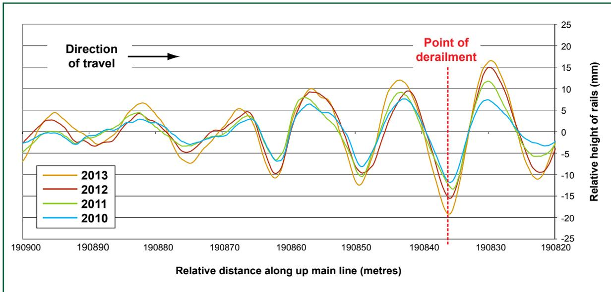
Figure 18: Track geometry recording data from 2010 to 2013
