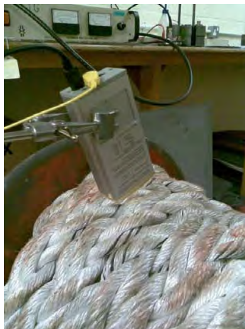
Figure 4 – Arrangement for measuring charge decay time from the rope.
