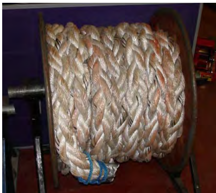
Figure 1 – Rope sample wound on to steel flanged core.
