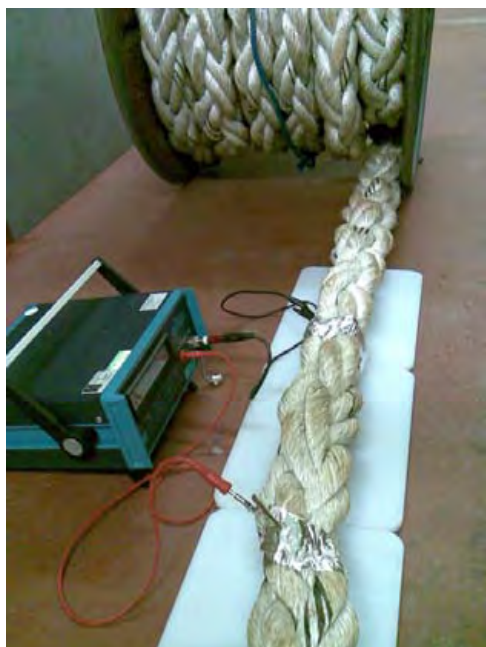
Figure 3 – Arrangement for measuring point-to-point resistance along the rope.
