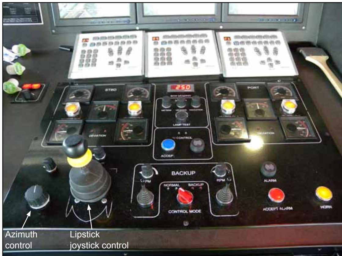
Manoeuvring station - Norman Arrow
