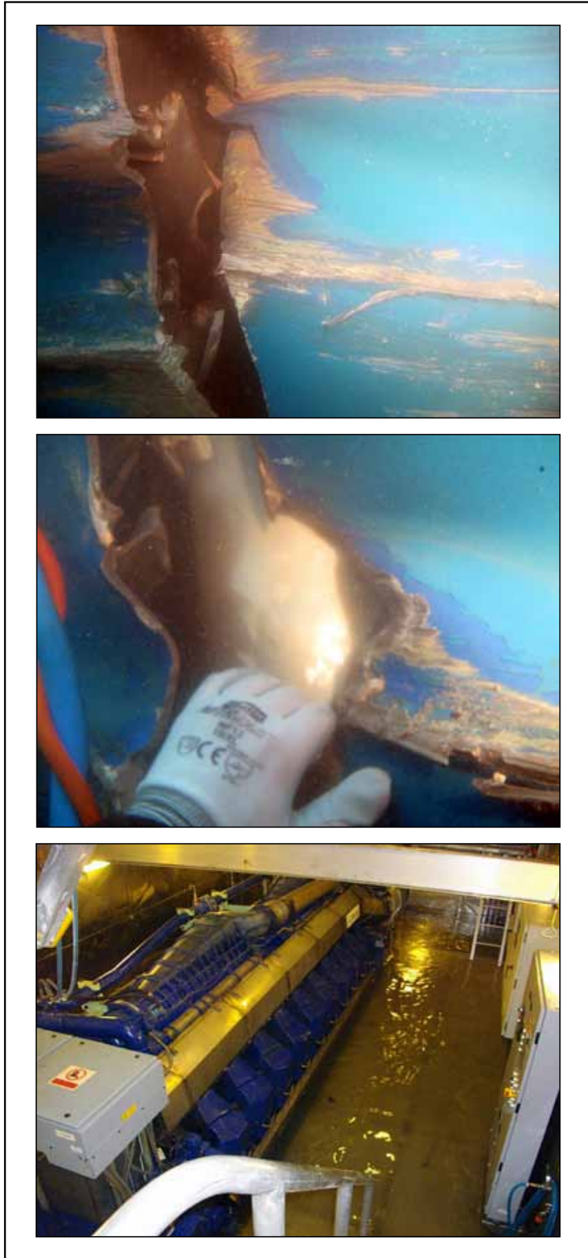
Norman Arrow hull damage and flooded engine room
