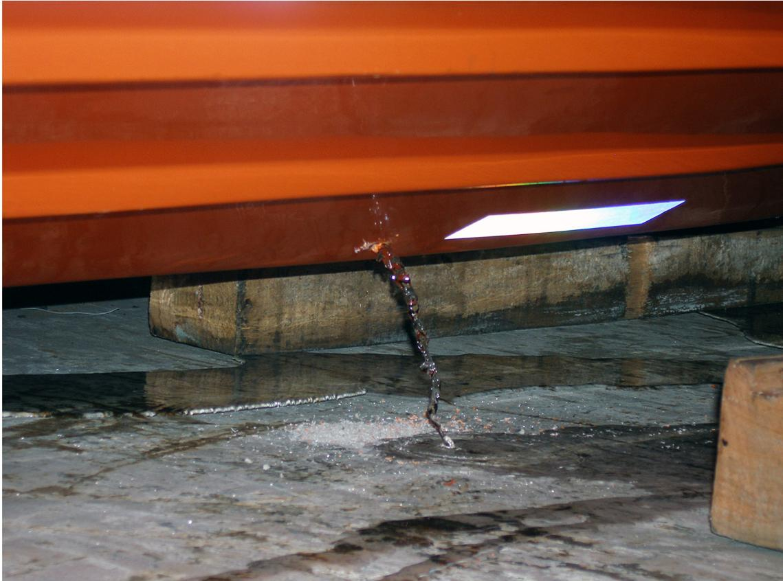
Water draining from foam-filled compartments
