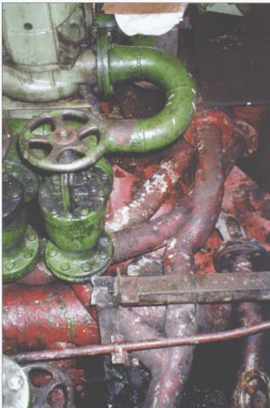
View of General Service Pump on sister vessel MV GREEN TULIP showing configuration of pipework below floorplates. The sea water inlet pipe to the G.S. Pump passed below these pipes.
