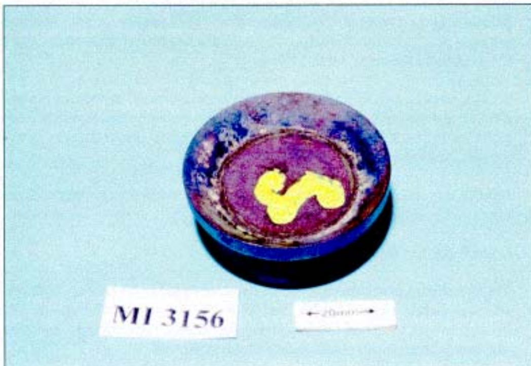
Figure 26 - Forward side valve cap, showing raised seating face, steam / water passing marks and associated deposits
