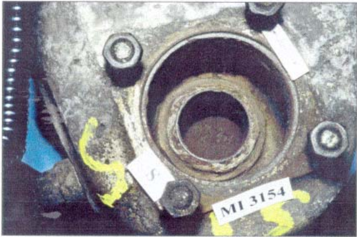
Figure 21 - Forward side valve seat and associated deposits
