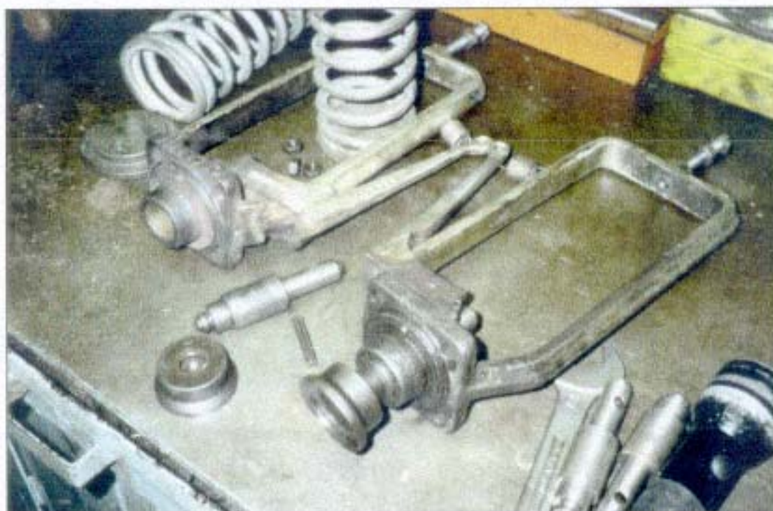
Figure 10 - Starboard safety valves
