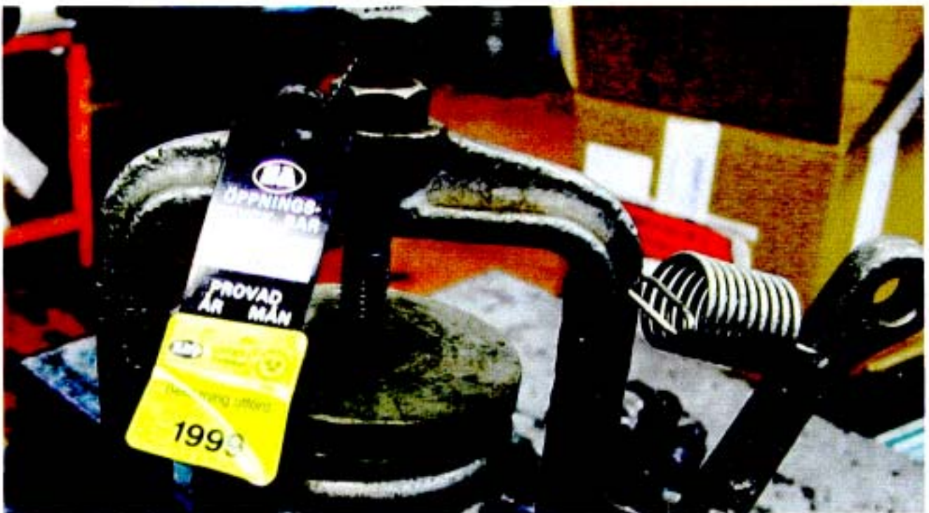
Figure 6c - Sealing arrangement for the NordAmatur safety valve (photo taken at the factory)
