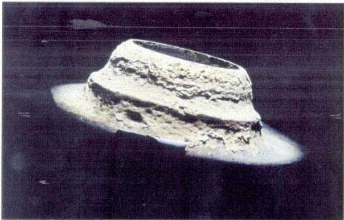
Figure 22 - Forward side valve seat and associated deposits
