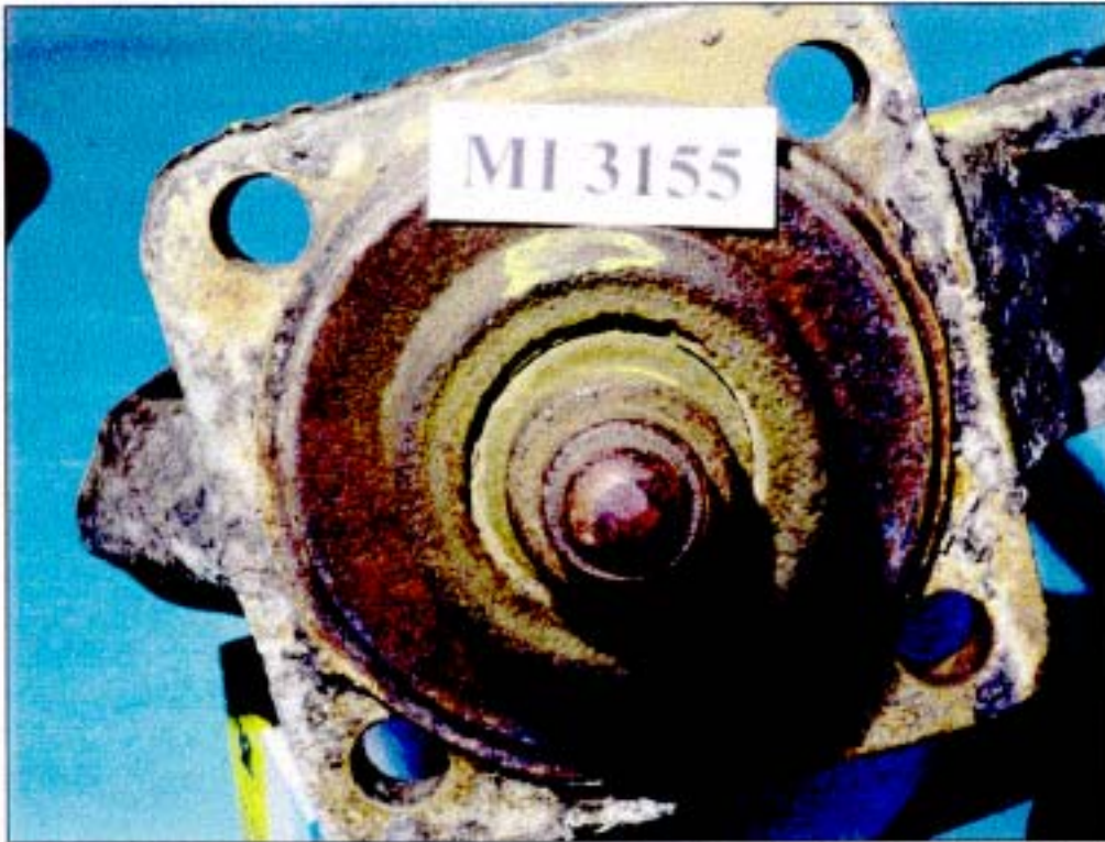
Figure 25 - Aft side valve lid underside and spindle, showing heavily oxidised hammer type marks at the spindle bottom
