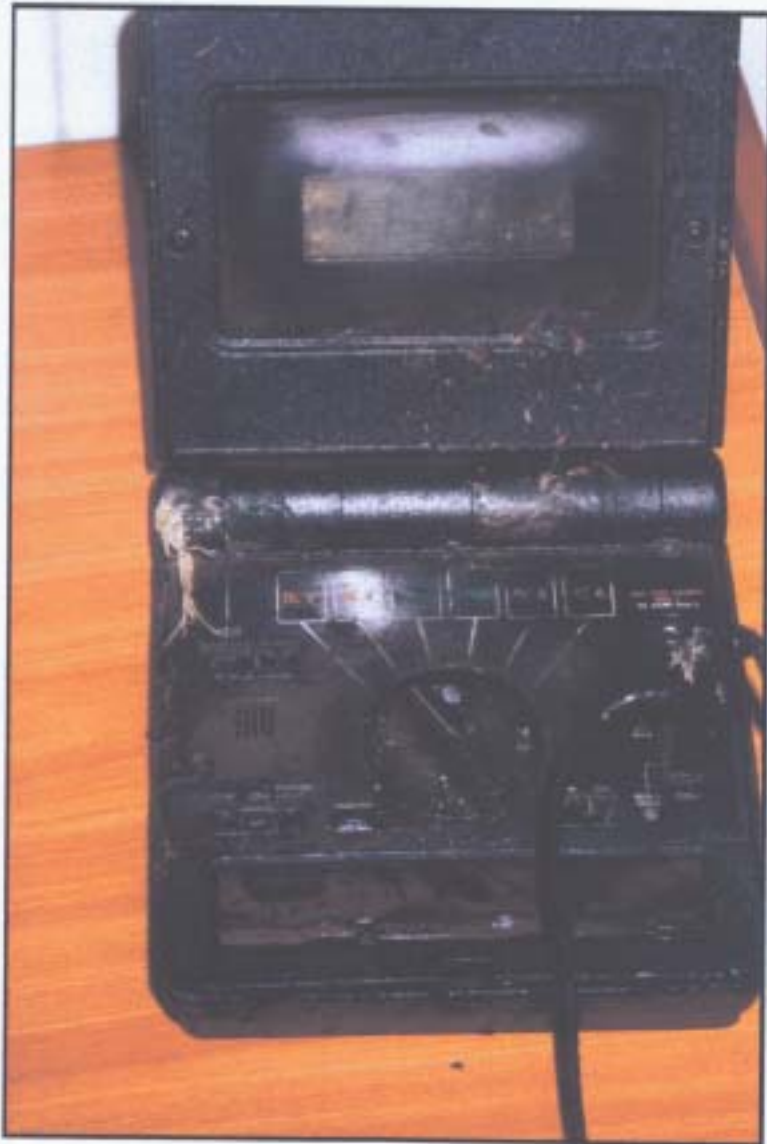
"Micronta" Multi-Meter condition after explosion. Note test lead in closed loop with meter set to measure Volts.
