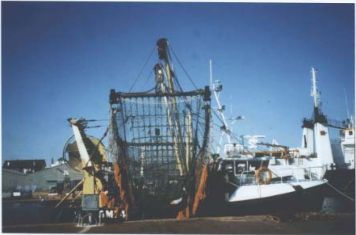
Trawl gear hauled aloft for repair
