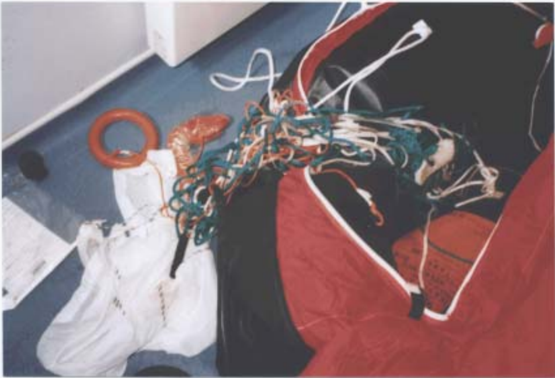
Figure 3 - Liferaft's quoit and line entangled with other equipment
