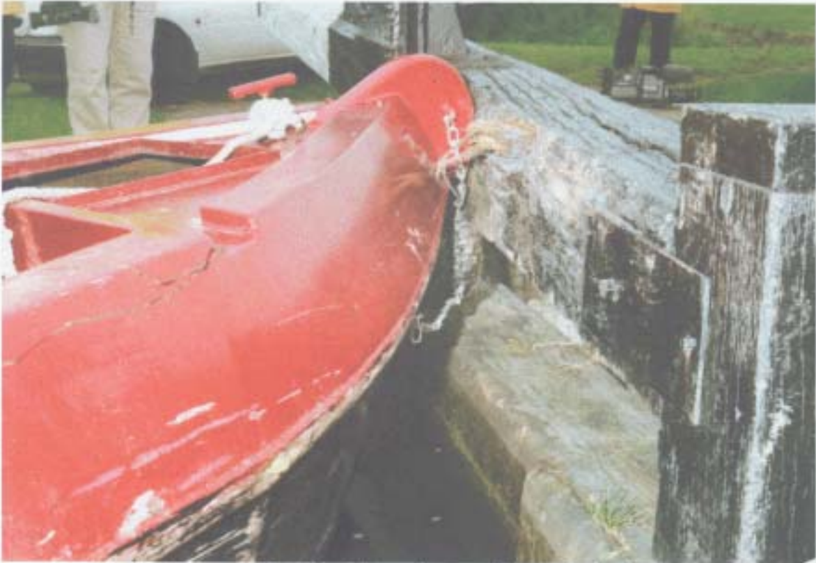
The snub nose against the balance beam with the fender in the gap.
