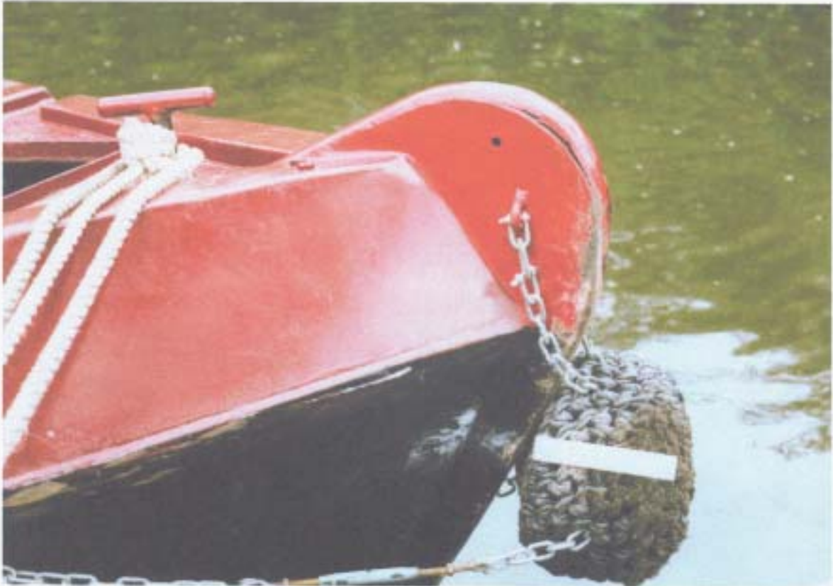
The Damage to the starboard side of the snub nose, which probably caused the splinter to the balance beam.
