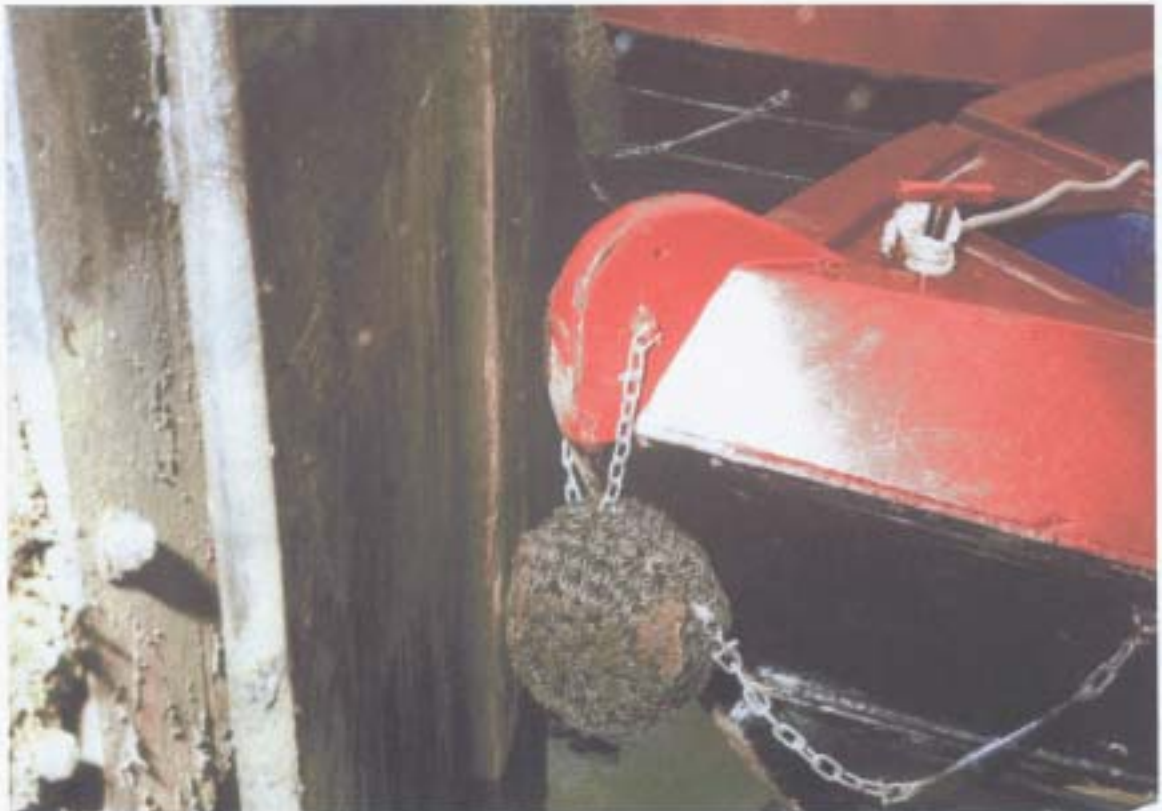
A view of the stem of DRUM MAJOR, showing the securing points for the fender chains
