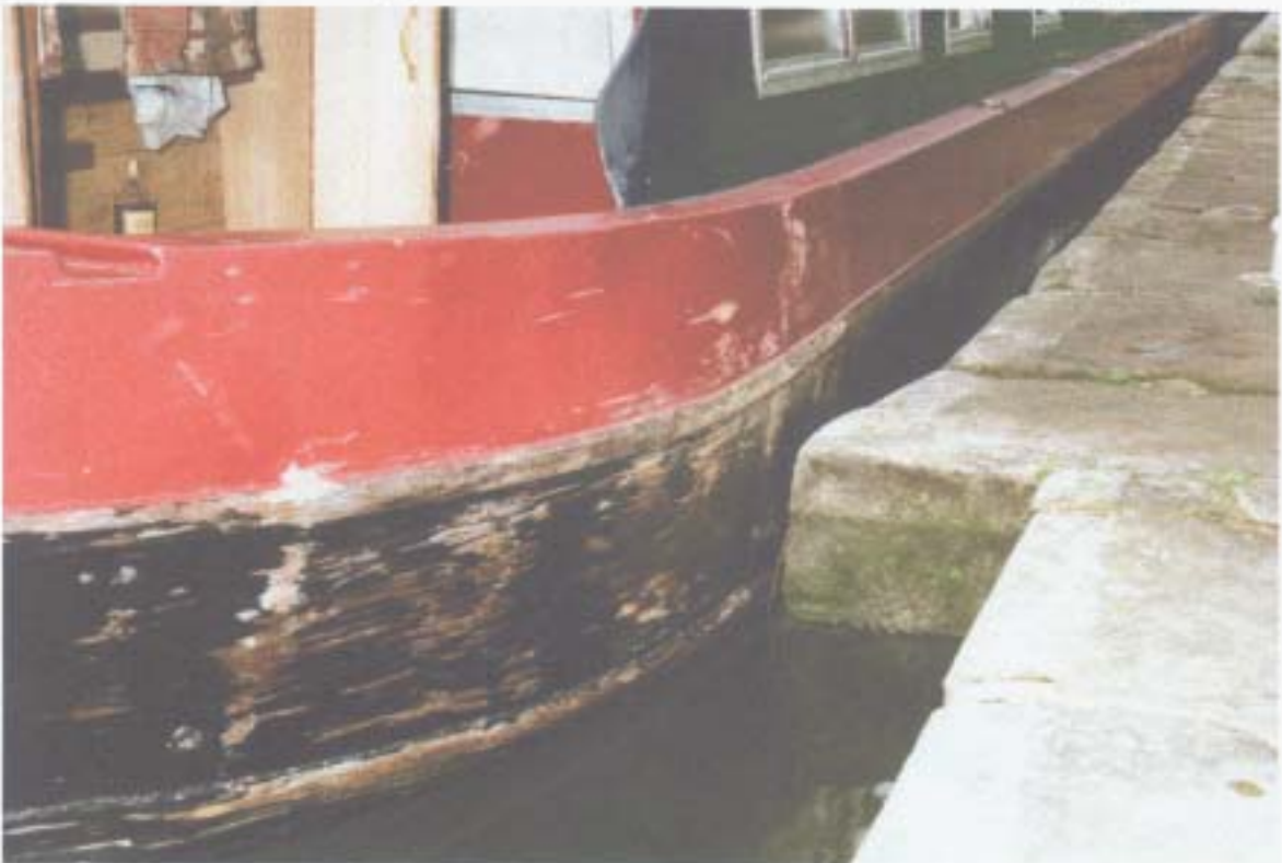
A view showing the port side rubbing bands in relation to the coping stones when the lock was full.
