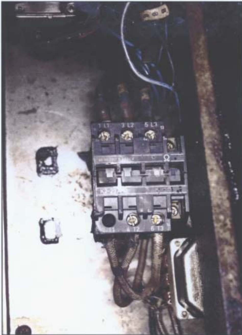
Figure 5. The contactor of the affected deep fat fryer.
