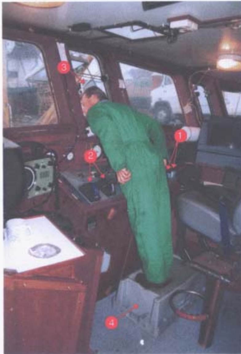
View of the winch control position in the wheelhouse
