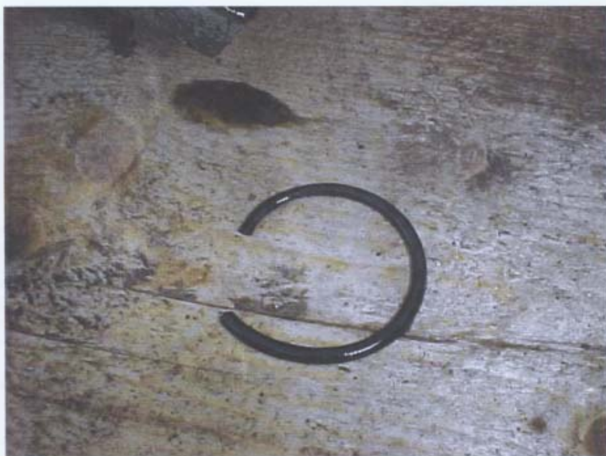
Broken seal ring
