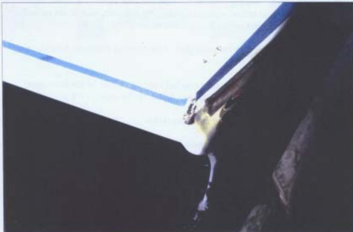
A view of the port bow corner of Beverley Ann II showing the slight damage to the GRP and the paint traces
