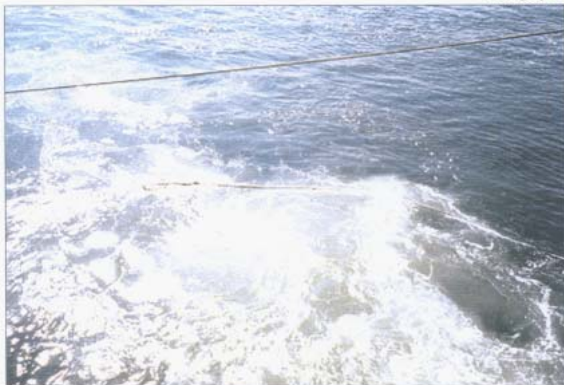
Mooring rope pushed away by astern propeller turbulence
