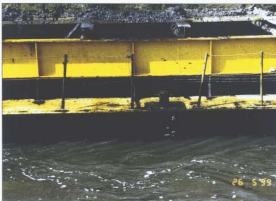
No 2 Close up view of starboard side of loaded barge. Note 5 foot draught (1.524m)
