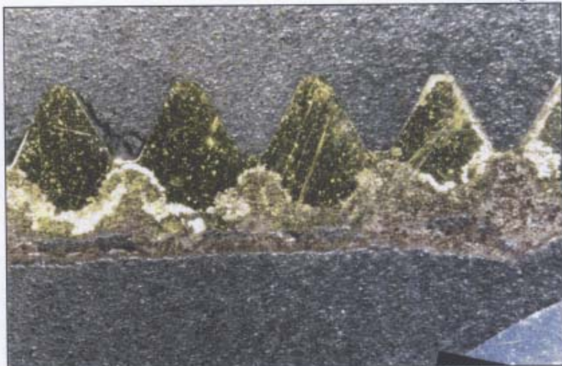
A section taken lengthwise through the wall of the failed fitting (magnification x 14.7)
