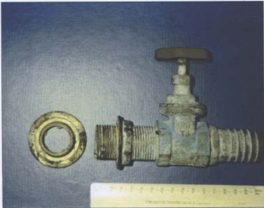
Random Harvest's failed through-hull fitting
