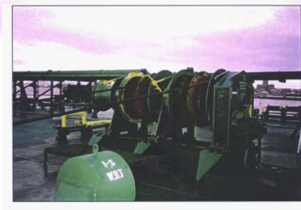
An overall picture of the starboard side forward deck-mooring winch
