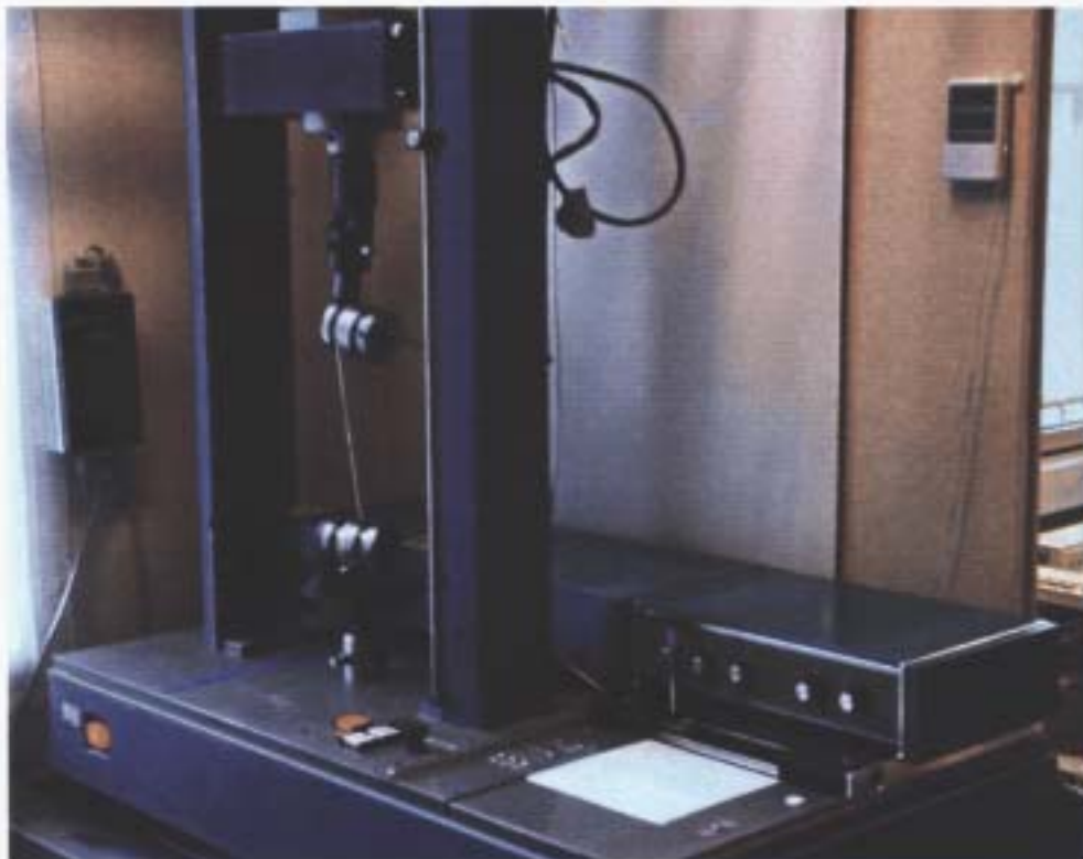
A yarn from the nylon tail undergoing a realisation test in Preston
