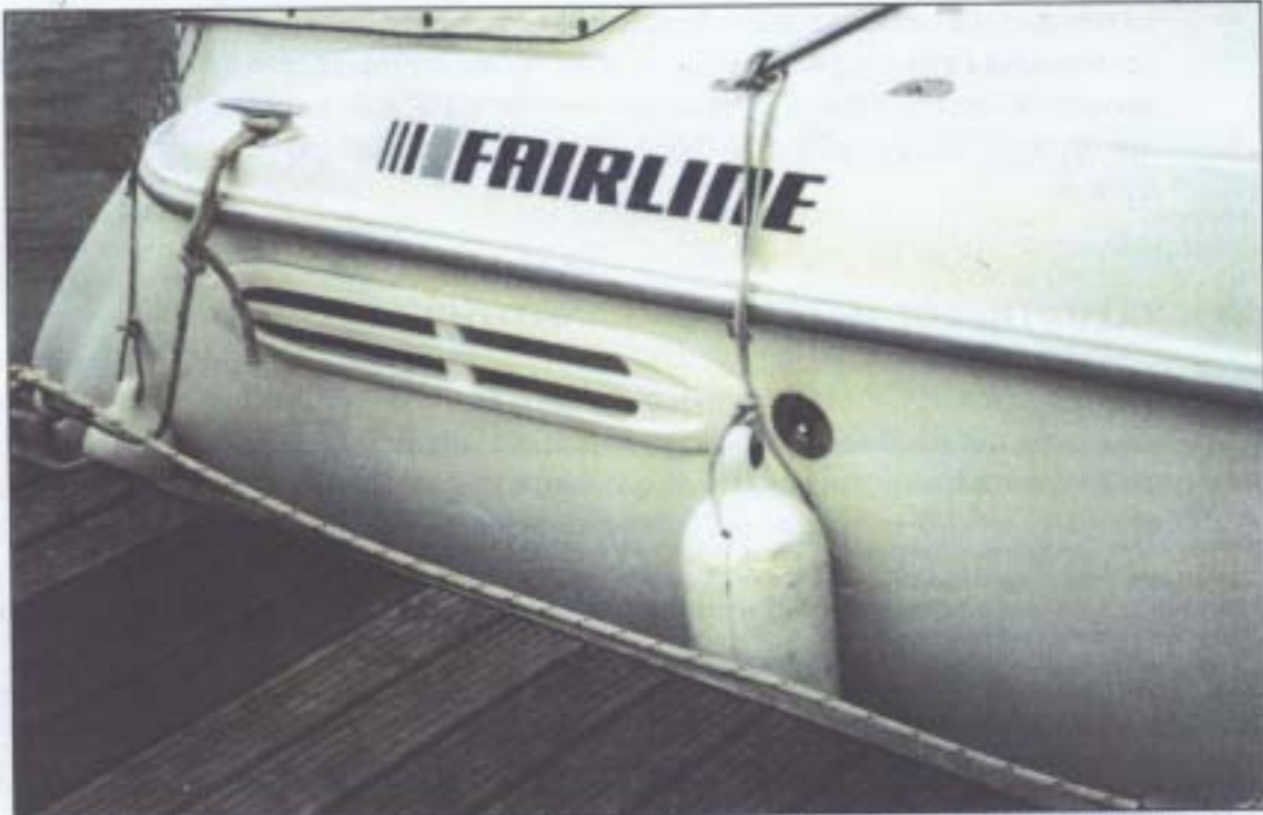
Diesel oil burner exhaust from cabin heater, forward of engine compartment air intake
