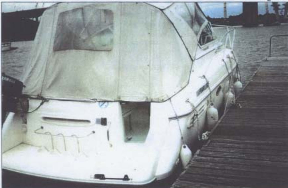
View from aft showing clear view panels on sides and aft of canvas hood
