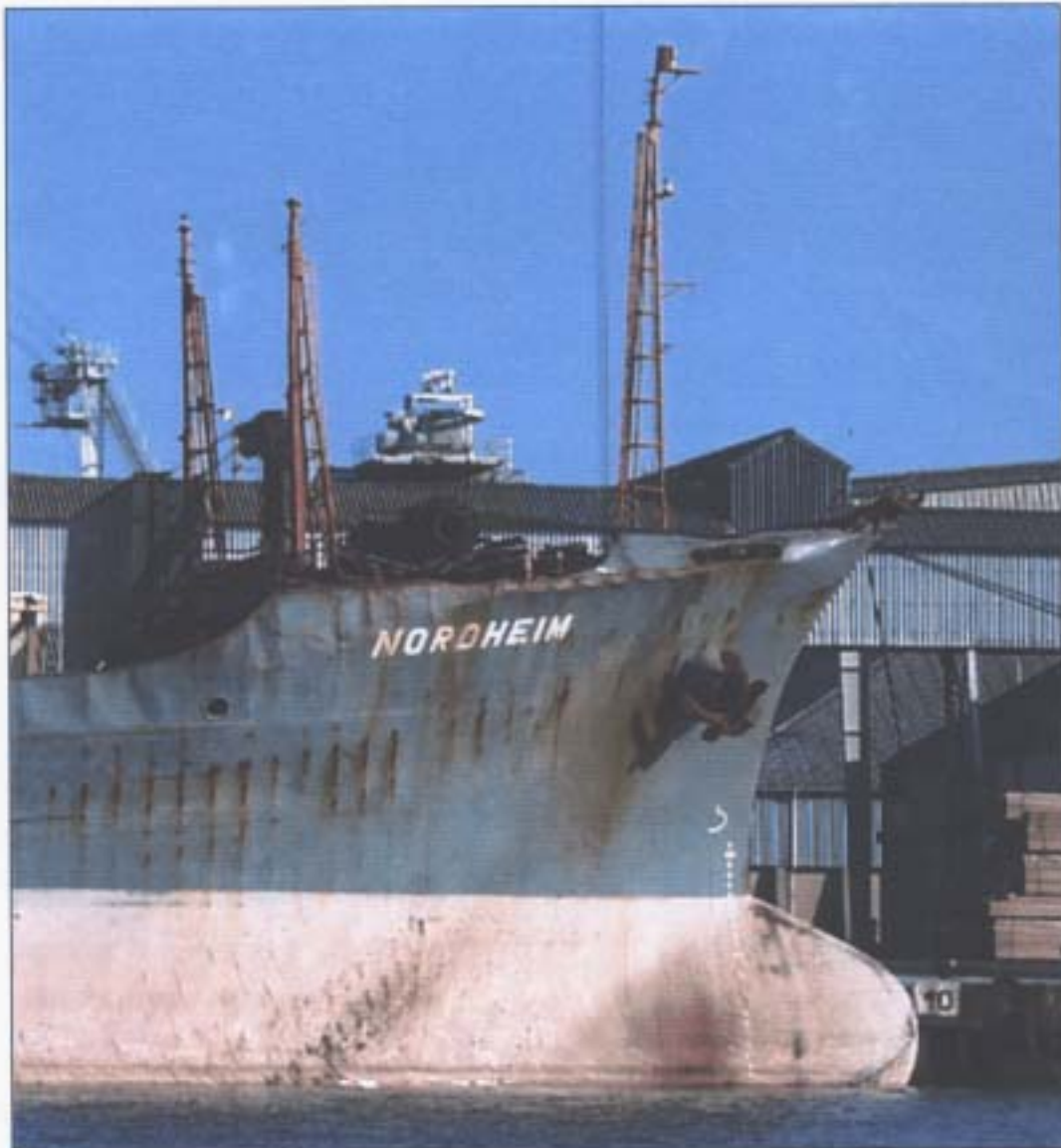
General view of Nordheim's starboard bow showing the damage
