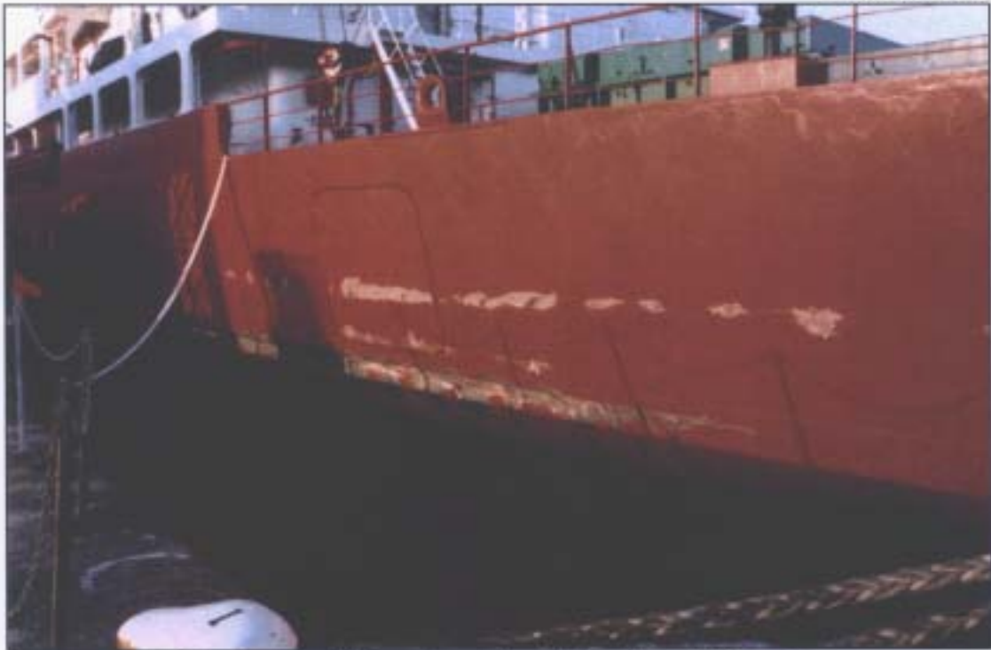
The damage to the port quarter of Pasadena Universal
