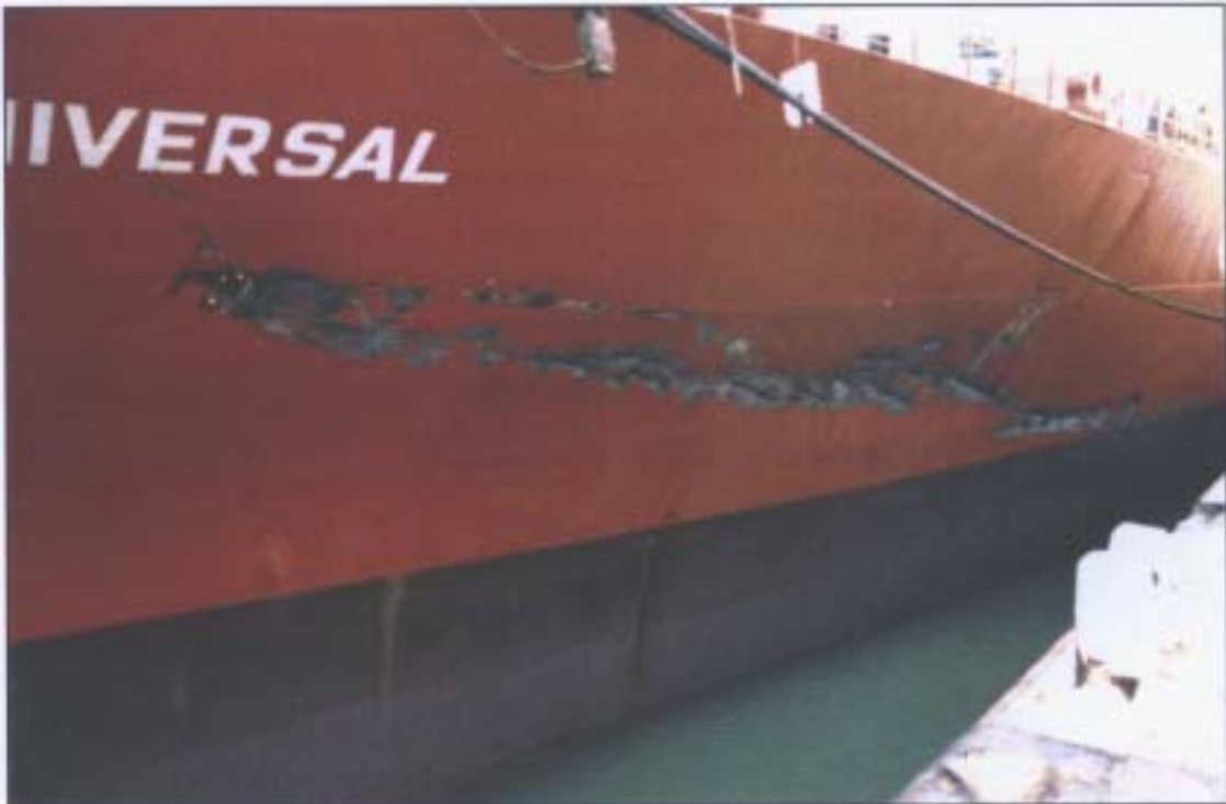
The damage to the port bow of Pasadena Universal
