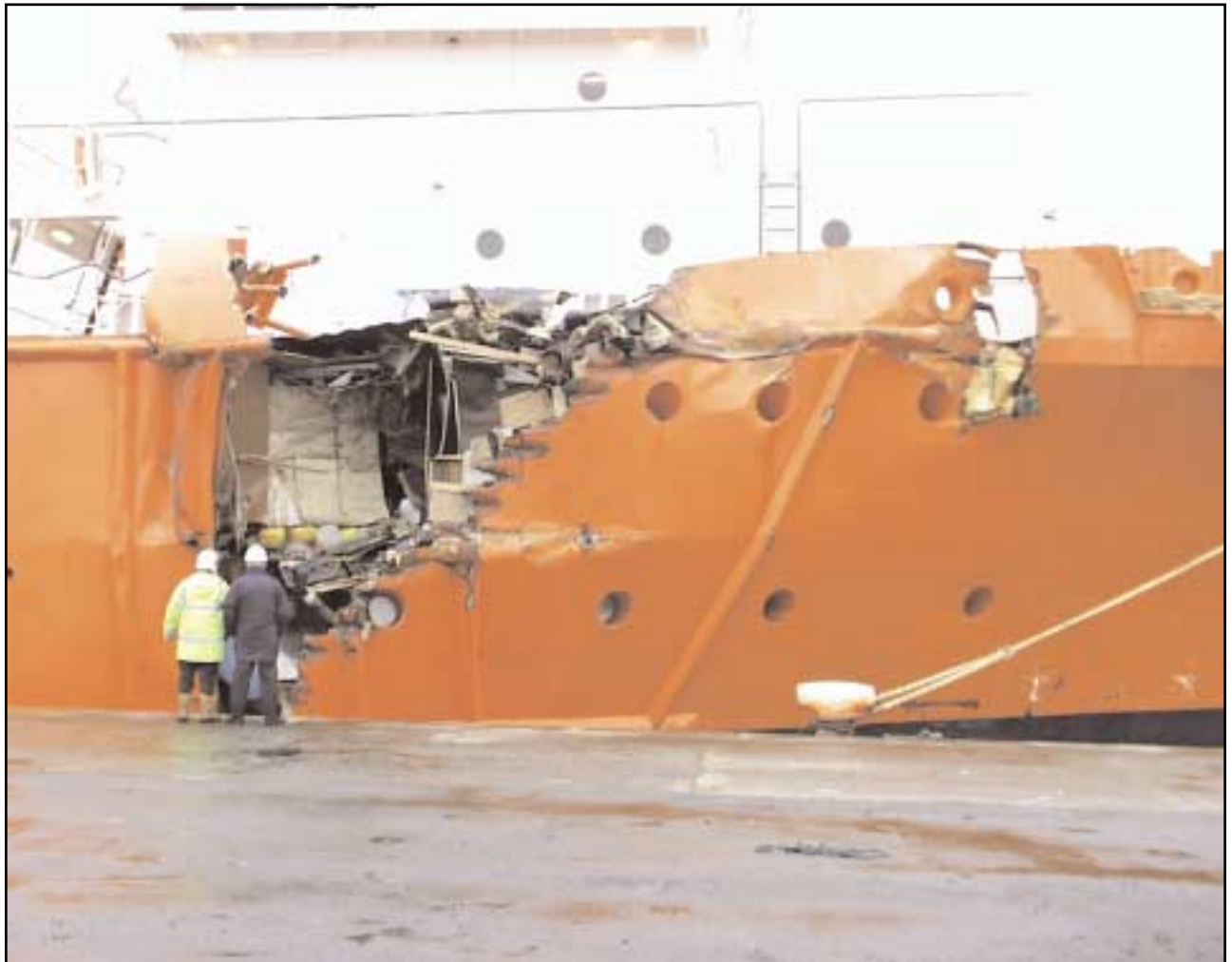
Starboard side forward. Side shell missing over a “V” shaped area from deck to waterline. Small opening in bulwark just aft of fairlead.
