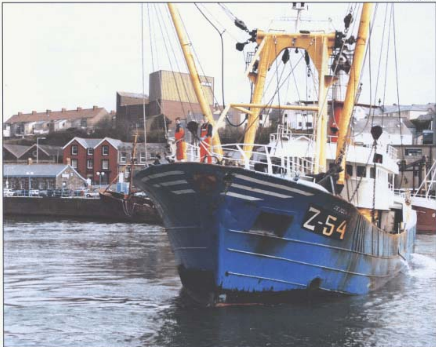
Damage to De Bounty confined to the upper part of the stem
