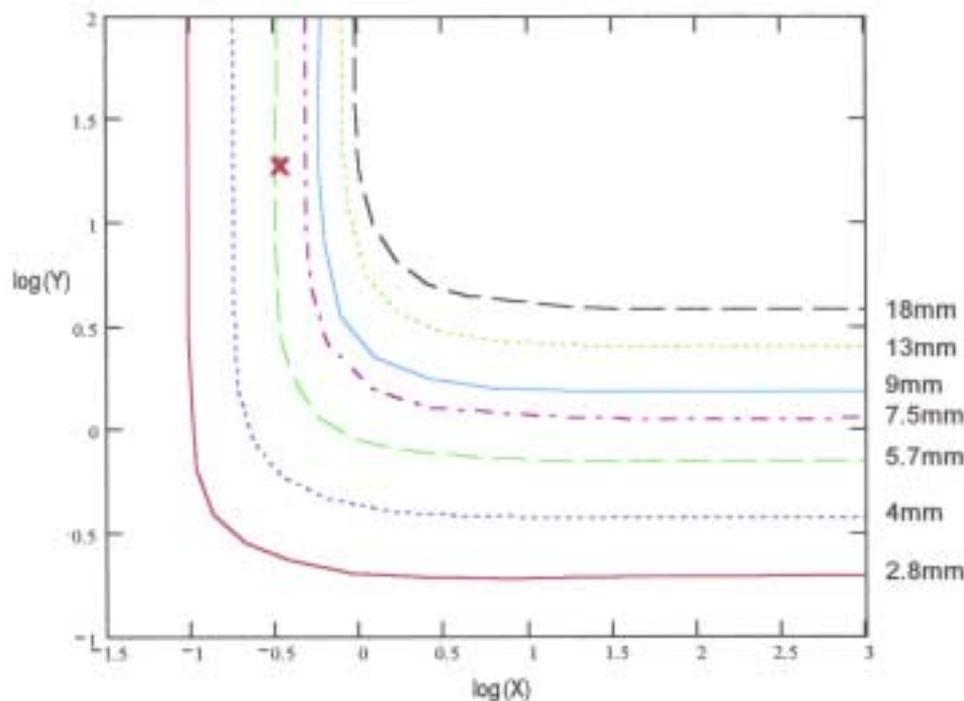
This result shows that the blast load would expect to deflect a hull plank by up to 6mm between the frames. This would apply to all the planks in similar locations.
