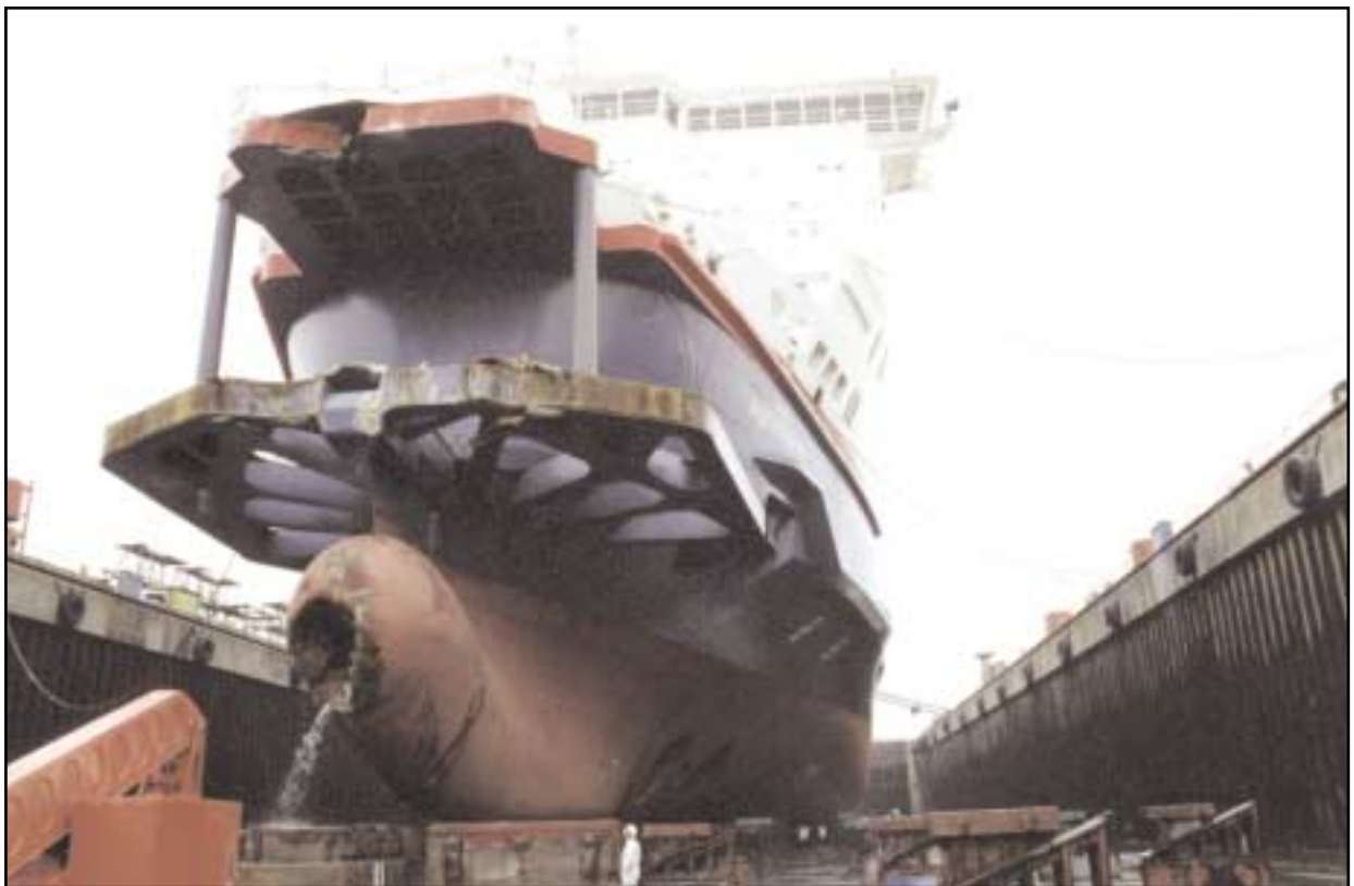
Damage to bow
