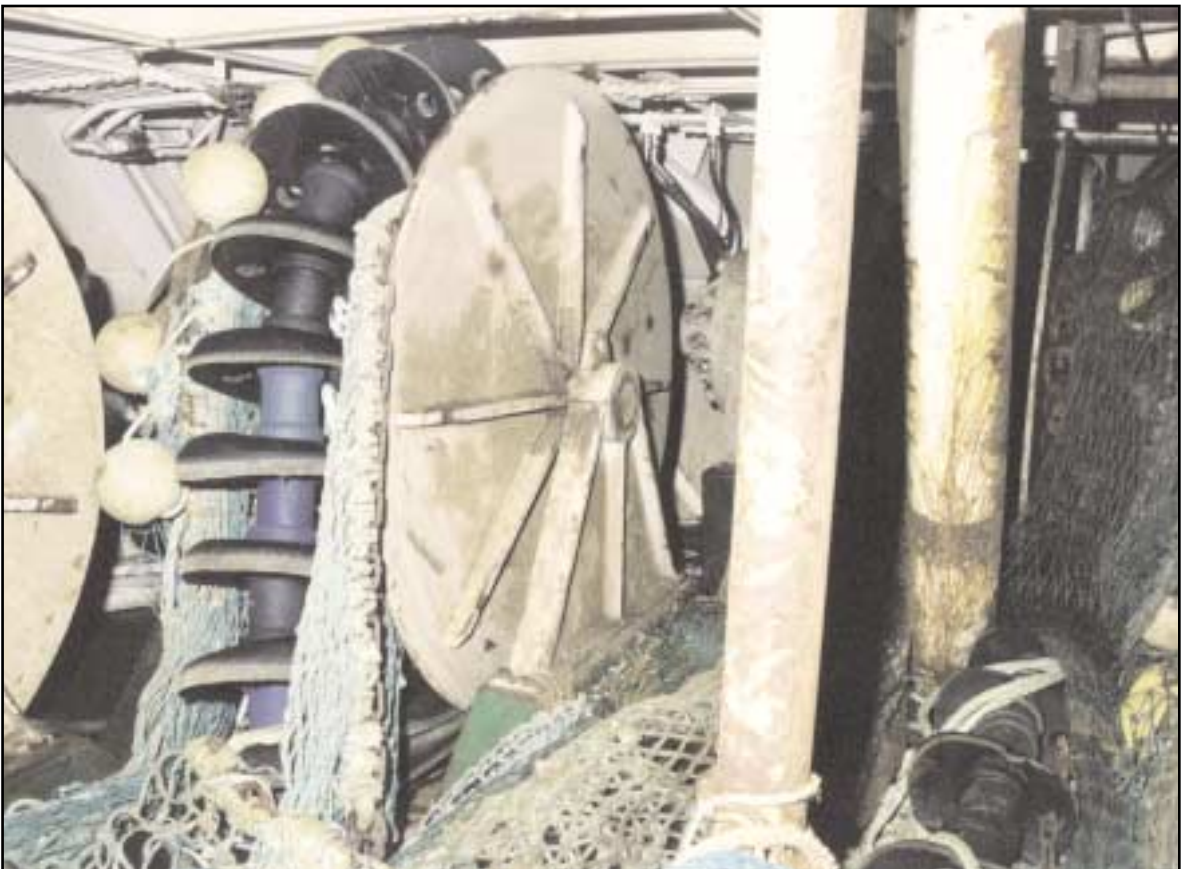
Inner port side sweep line winch
