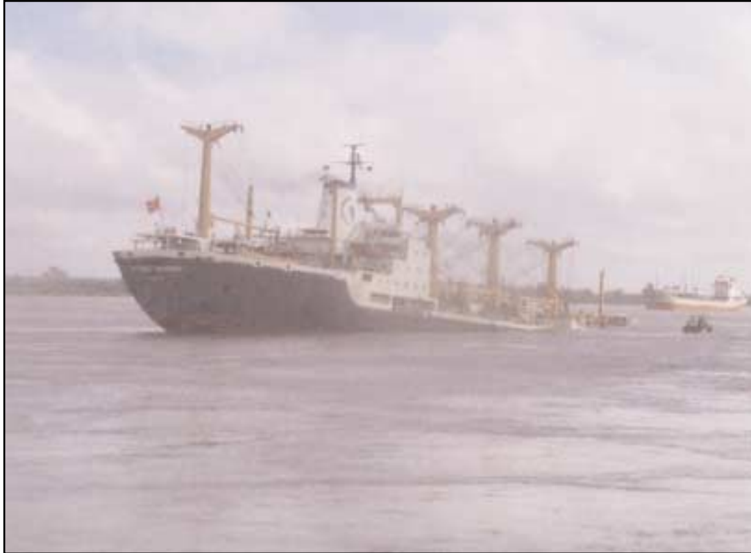
Flooding of Global Mariner following the collision
