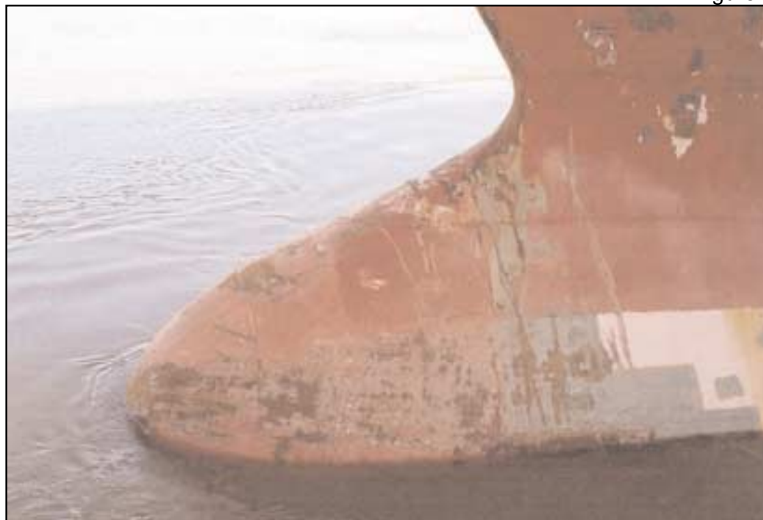
Bulbous bow of Atlantic Crusader after the incident
