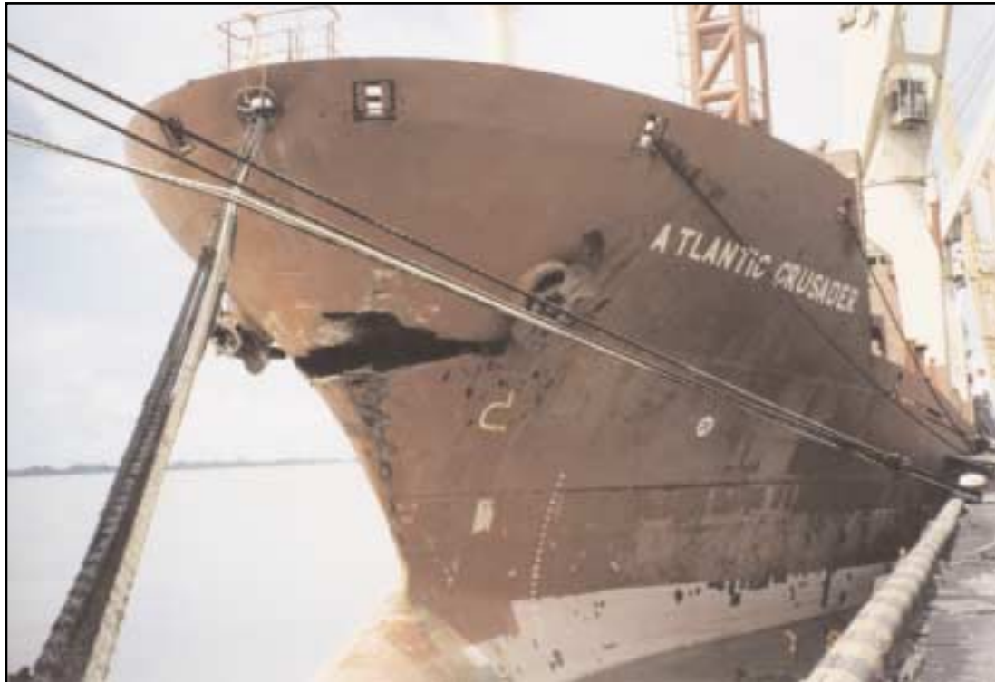
Damage to stem of Atlantic Crusader
