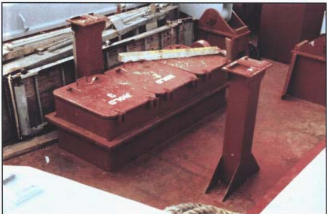
View of hold access hatches between holds 2 & 3 with deck cargo removed. Entry to No 2 hold is the middle hatch
