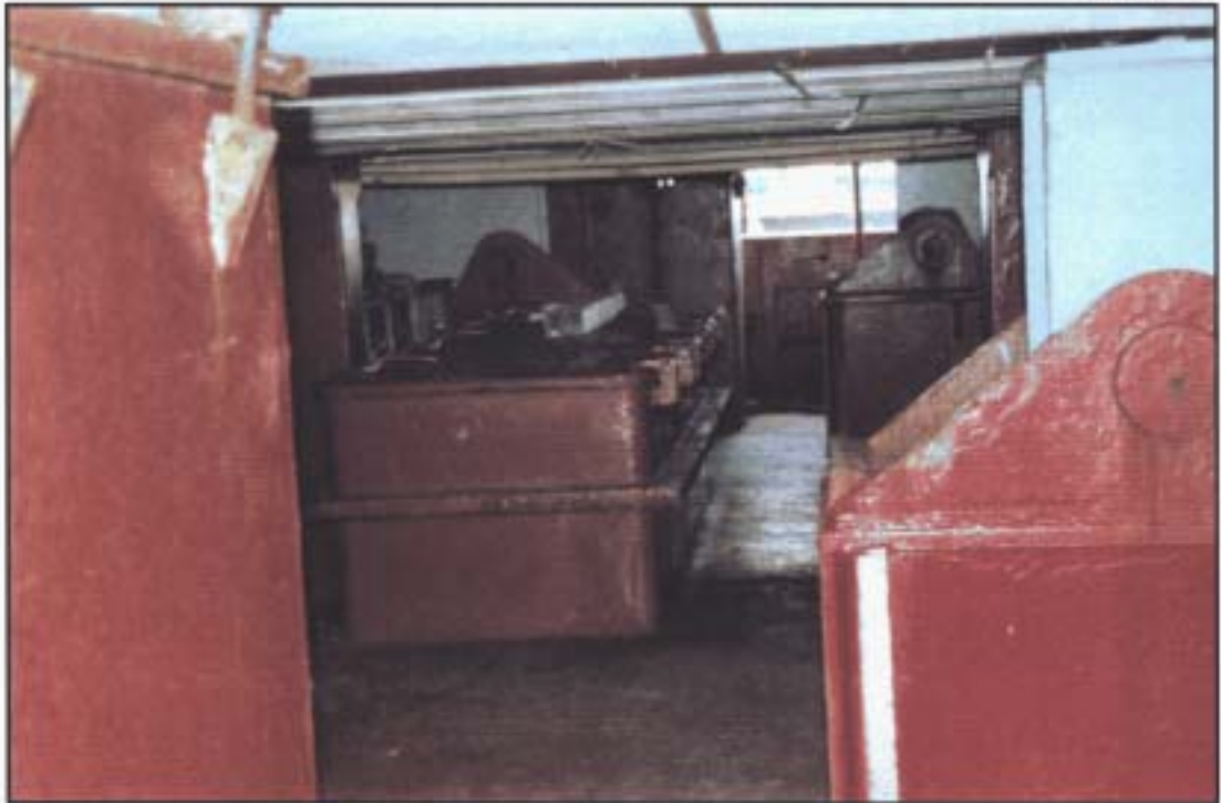
View of deck space between hatches 2 & 3 with deck cargo in place - note limited headroom
