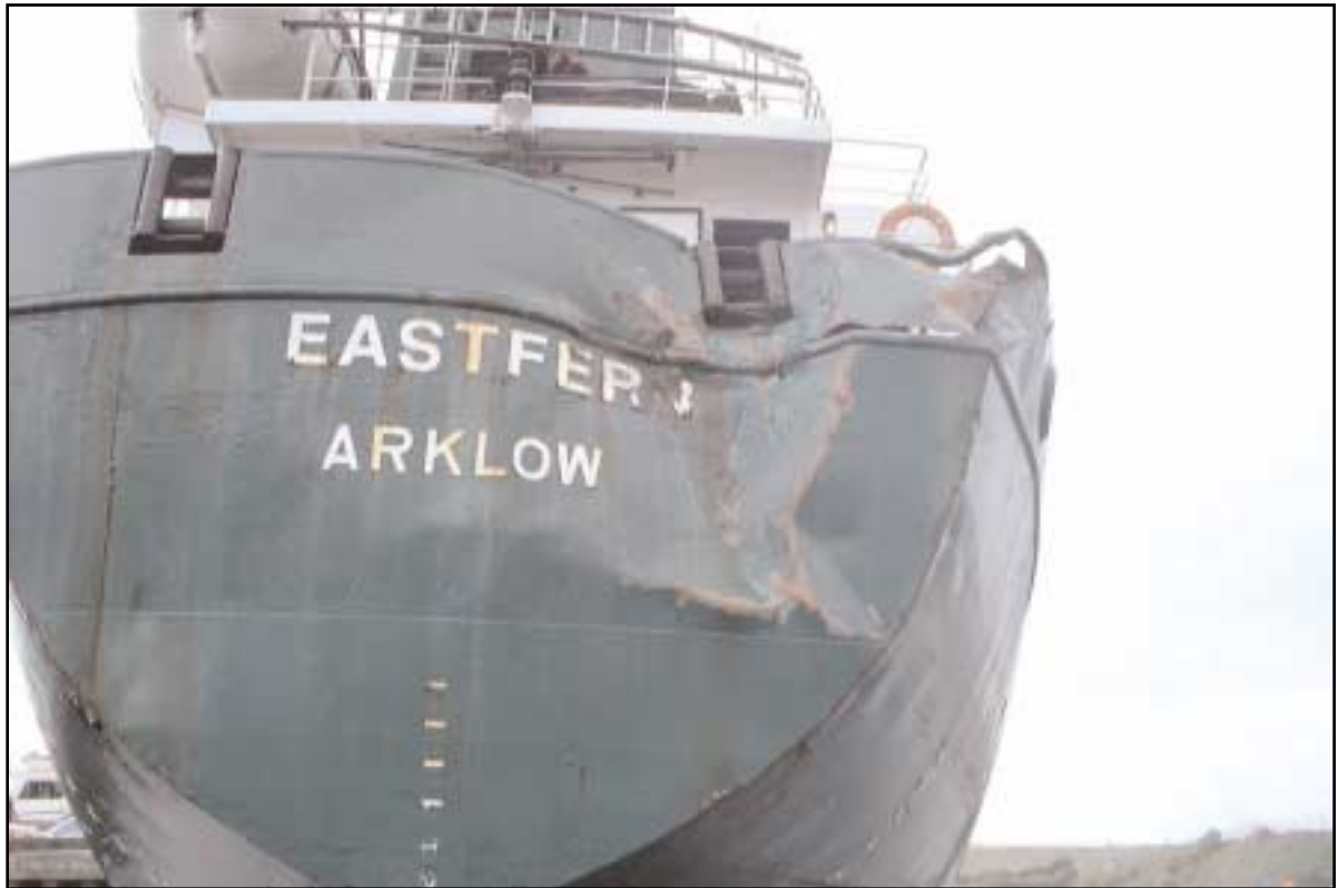
A view of the damage to the stern
