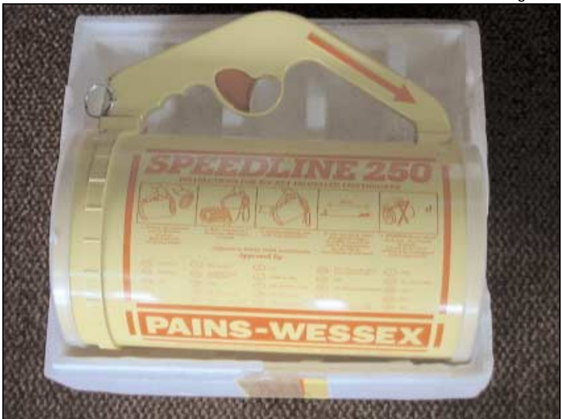
One of the four rocket line throwing apparatus units stowed on the bridge of Koningin Beatrix
