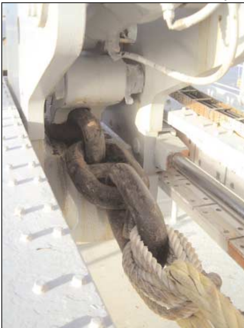
Chain stopper with hydraulically-operated claw in the locked shut position
