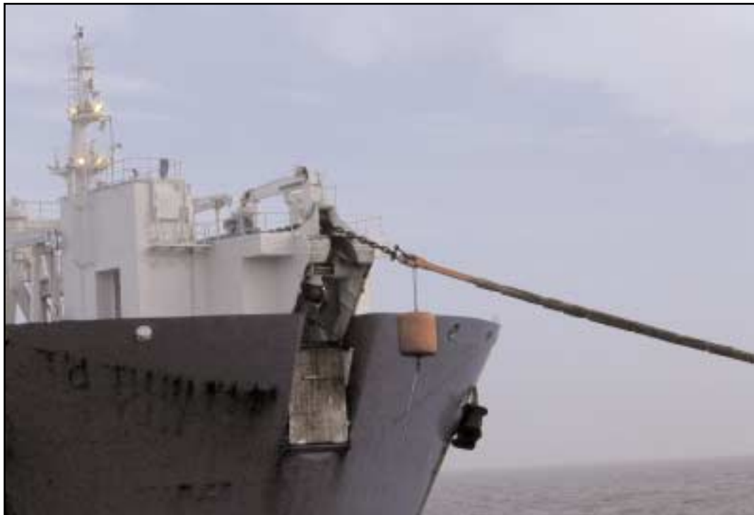
Vessel secured to buoy with hawser and chafing chain, the chain passing over bow roller and locked into the chain stopper
