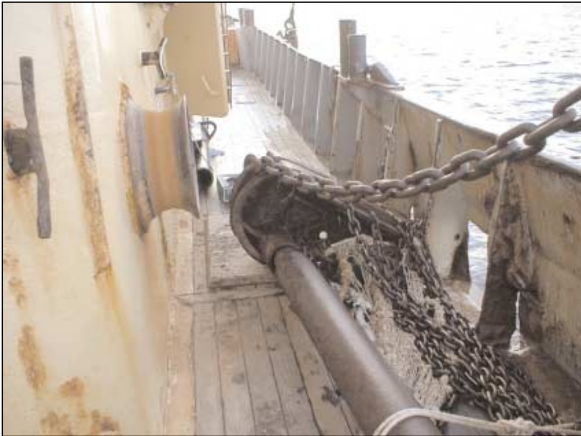
View from forward of the beam shoe having fallen onto the deck
