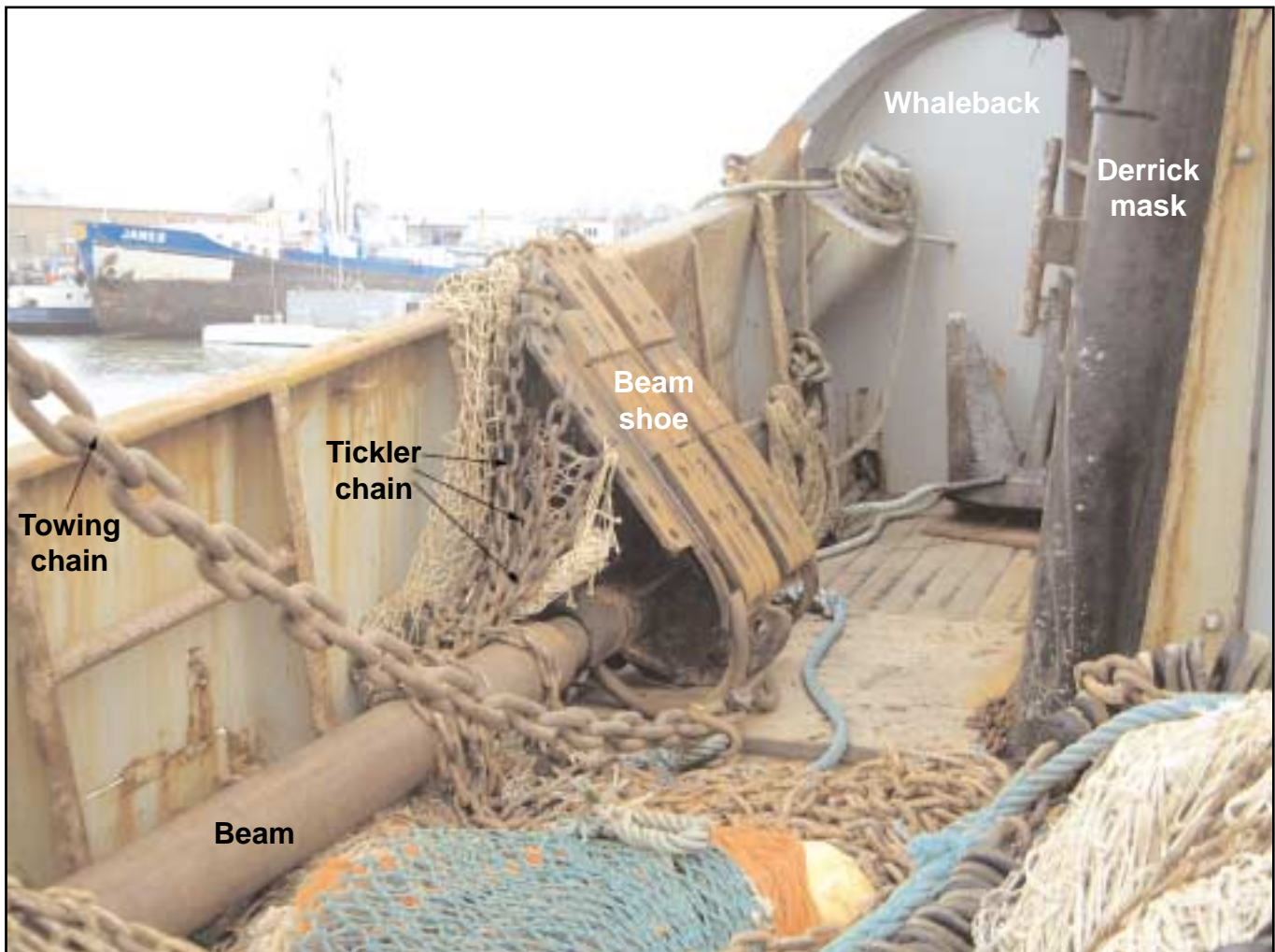
The forward end of the beam
