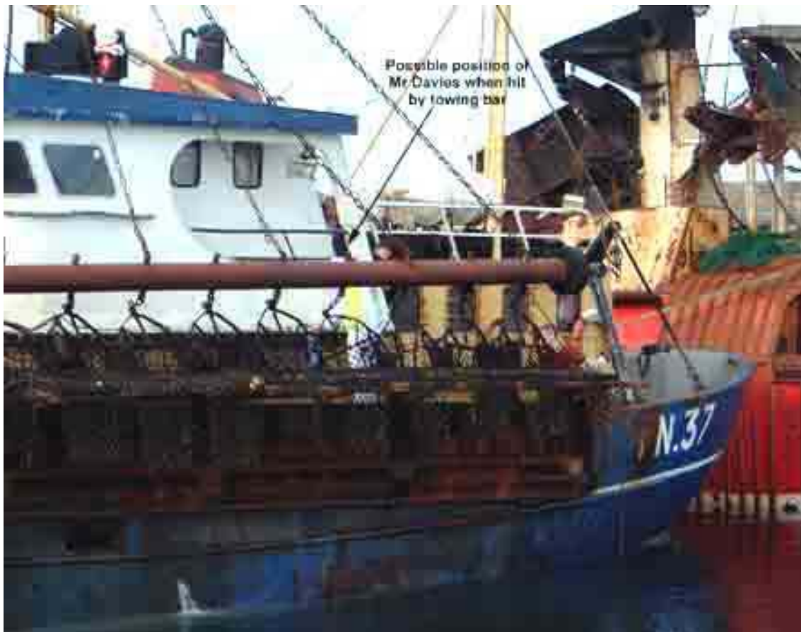
Estimated height of the towing bar and position of Mr Davies at the time of the accident Figure2
