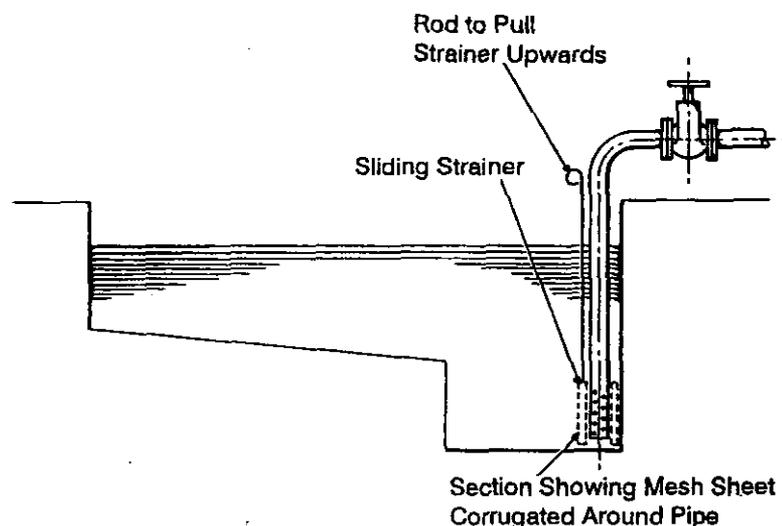
**Figure 5 - Sliding Suction Strainer**
