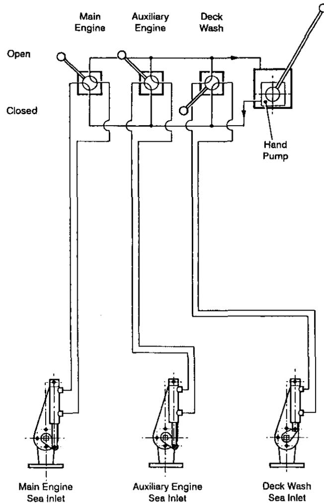
Figure 2 - Remote Operation of Seacocks
