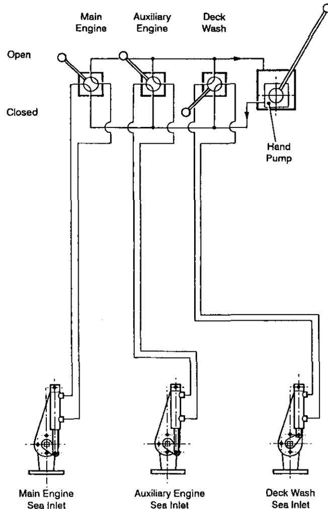
**Figure 2 - Remote Operation of Seacocks**
