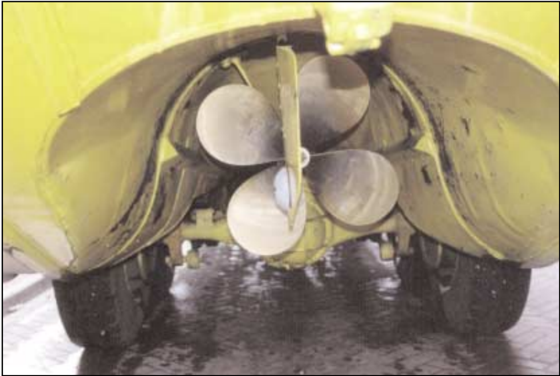
Rear of Beatrice showing propeller and rudder in recessed propeller duct
