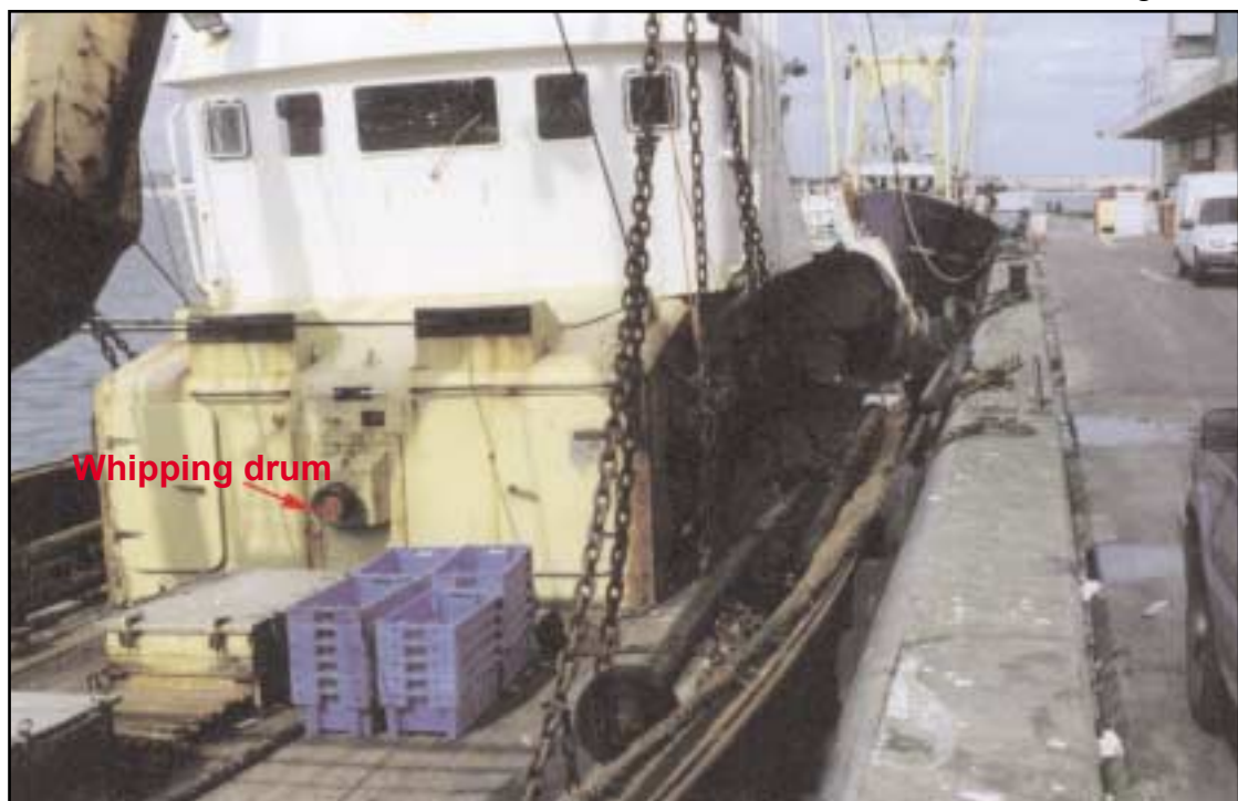
General view of wheelhouse and winch house. Note central position of the whipping drum (painted red).
